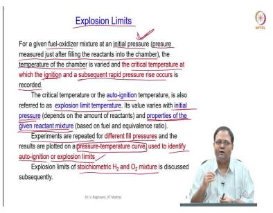
Now, so as I told you, this auto ignition temperature leads to a rapid pressure rise, rapid pressure rise and we call it explosion. So, this is also called explosion limit temperature; that is what we are going to see next, explosion limits.
