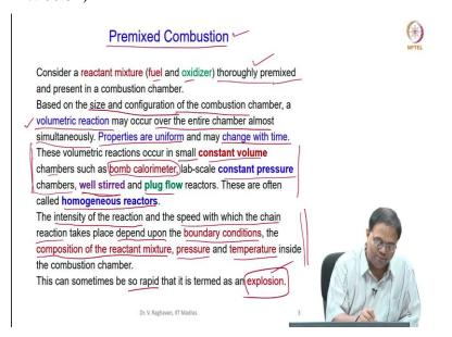
So, premixed combustion, consider reactant mixture that is fuel and oxidizer thoroughly premixed and present in a combustion chamber.
