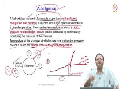
Now, let us see one more thing; see in the in these cases you know, normally we should have some ignition sources. Especially when the reactants are fed at the very low temperature so initially the reactant can be at temperature of 298 K.
