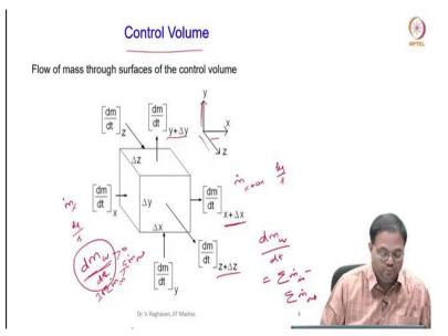
A control volume; so, you can see that control volume is shown here; as I told you we have taken the Cartesian coordinate. So, this is x direction here; x direction is horizontal direction, vertical direction is y direction here and z direction is the mutually perpendicular direction.
