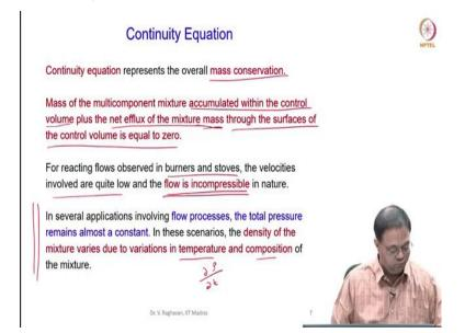
So, continuity equation represents the overall mass conservation; mass of the multi component mixture accumulated within the control volume, the transient term, the time dependent term + the net efflux, that is the outgoing mass flux - incoming mass flux of the mixture. So, net efflux of the mixture mass through the surfaces of the control volume is equal to 0.
