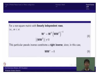
For example, you take a mecanum wheel 4 mecanum wheel drive so where n would be you can say  $\omega_1$  to  $\omega_4$  where n = 4, but you have  $\begin{bmatrix} u \\ r \\ v \end{bmatrix}$  in the sense 3. So, 3 is actually less than 4 in the sense what you can see the non square is exists. Here, what would be the maximum rank you can expect?
