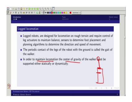
So, in that sense what you can see the periodic you can say contact of the leg supposed to be you have to monitor. So, that the periodic contact of the leg of the robot what you call gait ok. So, now the gait would be stable gait supposed to be. So, then only you can do. So, now you know like the human would be walking right, the human walking in one particular style that is what you call human gait.
