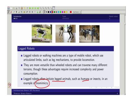
So, in that sense what is legged robot? Legged robot is what generally we call walking machines it is based on the legged locomotion. So, in the sense we have like artificial limb that would be act as the locomotive device. So, for example, you can see here it is a four wheel sorry four leg locomotion here, it is a two leg locomotion and it is actually like six leg.
