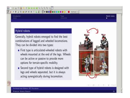
So, now what you can see? So, one subclass is what I call hybrid robot, so where the wheel and leg is connected. So, there are two way you can do it. So, what one actually like you can do? The leg is attached with the wheel at the end instead of having a foot, you can actually like put the wheel. So, then this is one class, so the other class is actually like you have two independent, so whenever you want you can actually enable it.
