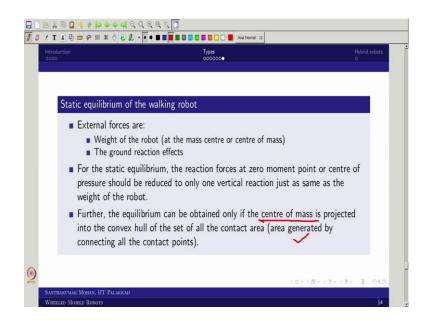
So, that some time we call center of pressure. So, then you can actually like bring the static equilibrium again. So the external forces what? So, one would be the body weight because it is static right, so, only the body weight and the support reaction. These two suppose to be neutral where? At the zero moment point. So, that is what we are actually like seeing these 2 forces are there.
