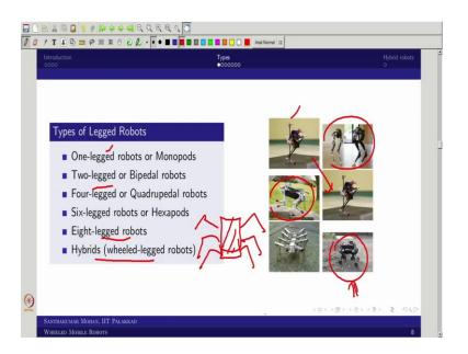
So, how that would be achieved? That we will see. So, before that you know the legged the robot can be classified in several form. So, we are classifying the legged robot based on the number of leg. So, if it is one leg like this it is what we call hopping robot we simply call monopod, pod means actually like leg, so, it is monopod means single leg, ok.
