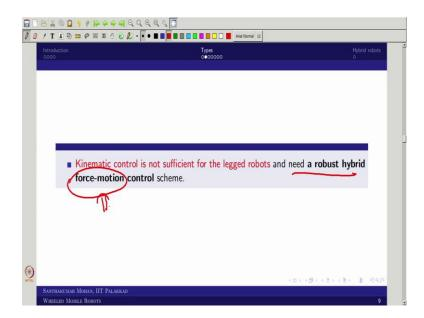
So, let us actually like move further. So, what would be the biggest challenge in the legged robot? You know wheeled mobile robot can be controlled in kinematic level, that is what most of the people are doing in mobile robot in general wheeled mobile robot. But that is not sufficient in the legged robot, why? Because, the stability is supposed to be ensured right, so, one of the easiest thing you take a pen so where it is actually like standing?
