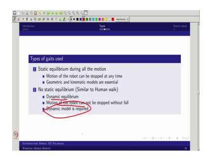
So, now the types of gait use actually like we are thinking about the static equilibrium gait. So, in the sense we are trying to duplicate as what the animal does, so try to duplicate and try to do it. So, in the sense motion of the robot can be stopped at any time if I am thinking about static gait.
