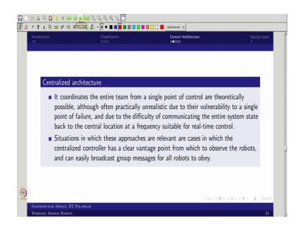
So, we will see what would be the centralized architecture. The centralized architecture one, issue or one important thing is it is a single point control. So, wherever it is actually like necessary, you have put it a single point control. So, for example, the group of robot, all the command is coming from the single node.
