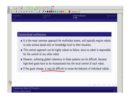
So, now we come to the decentralized architecture. So, it is completely decentralized right, this is the most common approach in multi robot because it is easy and you can actually like dictate individual task and it is actually like robust to failure, but the problem is actually like no robot is responsible that is the problem ok.
