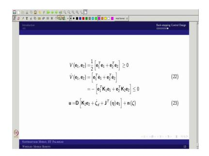
So, these two relations you substitute in this equation and that will give you can say the negative definite ok. So, in the sense what one can see the closed loop stability also ensured. So, now, what you can recall this equation? So, where you have substituted this right. So, this you recall. So, what is  $e_2$  2? So,  $e_2$  is actually like  $x_{2d} - x_2$ . What is  $x_2$  is
