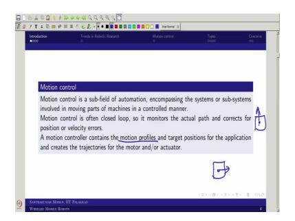
So, that is what we are trying to address. So, in the sense what you are trying to give? So, you would be giving a motion profile and some of the target position. So, this particular robot supposed to follow that some cases the trajectory also you need to create for your given motor or actuator or sometime even you have to create a trajectory for the robot.
