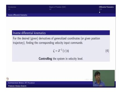
So, in the sense you are trying to do the reverse way. So, that is why it is called inverse differential kinematics, where you can see that for a given you can say it desired derivative of generalized coordinate you are trying to find out, you can sees that corresponding velocity input command.
