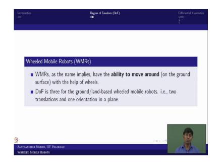
So, in the sense what we are doing in this particular course? This particular course is all about wheeled mobile robot. In the sense, I am putting the same keyword again. So, ability move around with the help of wheels. So, in the sense the degree of freedom in this case is 3, right. So, now, two translation and one orientation we need to describe in a plane.
