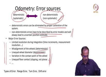
So, this is something which we need to reduce, but reducing this one I already mentioned about the error sources. We will be having deterministic sources and determining errors and non deterministic errors. So, these deterministic errors can be eliminated by calibration, but non deterministic errors need to be modelled by some methods. So, we use the probabilistic model as I mentioned earlier. So, we need to use the probabilistic model and then use that one to model the non deterministic errors.
