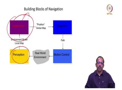
So, localization basically requires the perception to be done. So, basically the sensors will go and create get the data, sensors will collect the data and that data will be processed with the information available with the robot either the map is given or the map is created and based on that it do the localization that is what actually happens in the robots.
