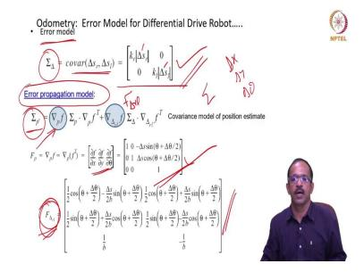
So, the  $\nabla f$  is obtained. So, this Jacobian Fp for the position estimate Jacobian we can get it as  $\nabla f$  which can be obtained by taking the partial derivative of f with respect to x y and  $\theta$ , because f is a function of this x y  $\theta$ . Therefore, we will be able to get this as partial
