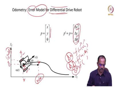
So, let us look at the error model for differential drive robots. So, we know that suppose, the robot is at this position. So, you have a robot and the robot is having two wheels as you can see here. Now, we need to develop a model for localization of these robot and we need to know how the model, the error in the estimated position will vary, because of the error in the encoders, because we will be using encoders to estimate the position of the robots.
