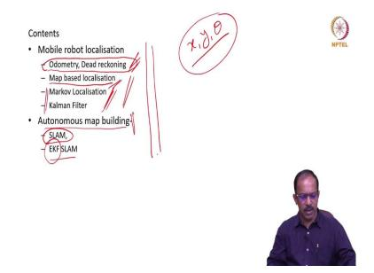
Now, in order to do that we need to understand few things that is basically how do the robot do the localisation ok. So, the first one to do localisation method is basically the odometry or we call it as the dead reckoning, that is the robot uses its sensors available on the robot and get the position and orientation and that is basically known as the odometry based localisation or a dead reckoning based localisation.
