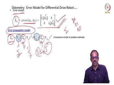
To do this, we need to look at the error propagation model. So, the error model for the sensor, we said that the sensor has got a error and that sensor error can be actually represented as a covariance  $\Delta S_r \Delta S_l$ . So, we assume that the covariance in sensing the
