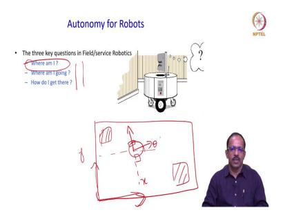
So, as I mentioned in one of the classes, autonomy for robots comes with lot of challenges and as I mentioned, the important requirements are the robot need to know where is it and where is it going and how would how can the robot reach there. So, these are the three questions the robot needs to answer. And the first question is where am I? And that can be answered through localisation.
