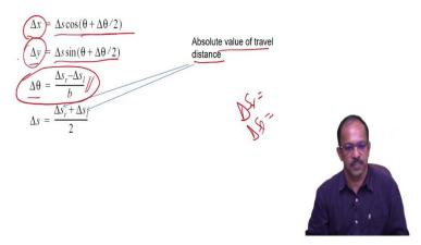
So, if you have this kinematics known. So, we know that  $\Delta x = \Delta scos(\theta + \Delta \theta/2)$ ,  $\Delta y = \Delta ssin(\theta + \Delta \theta/2)$ , and  $\Delta \theta = \frac{\Delta S_r - \Delta S_l}{b}$  and  $\Delta s = \frac{\Delta S_r + \Delta S_l}{2}$ . What is  $\Delta S_r$ ? They are the absolute value of travel distance.
