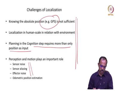
So, there are many challenges in localization as I mentioned, because the robot needs to know its local position not an absolute GPS position is not sufficient. GPS says that you are at this particular latitude and longitude that it is not sufficient for the robot. The robot needs to know within a room or within a human environment where it is that is the information with reference to a particular frame.
