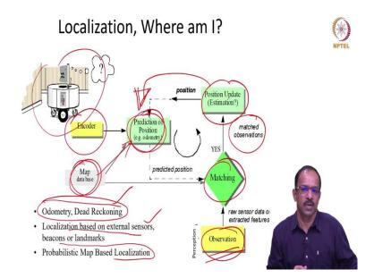
So, if the robot is moving in the environment, it will be having its own encoders. So, the using the encoder data we can actually use the odometry to get the localization done that is the primary localization. So, it will predict the position of the robot using odometry and then it will be having a map given to this assuming that, that map is given, then it will check with the map this one and then see what is the predicted position if the mapping features are known.
