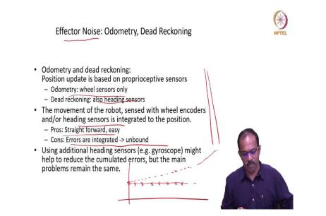
So, these are all challenges in using sensors for localization. And of course, there will be noise from the effector that is the actuators; the motors will be having their own errors. Though we have many things that the wheel encoders and or heading sensors when you integrate it may be easy to do this dead reckoning, but there will be lot of errors, because errors are getting integrated unbound.
