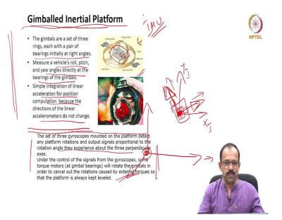
Now, how do we actually place this inertial sensors? So, there are two ways of doing it. One is by placing the sensors the sensor on a gimballed inertial platform. This is where you identify the orientation of the sorry identify the axis of the robot and then you have a inertial coordinate frame also. So, you have a fixed frame and a mobile frame.
