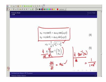
So, like that I can write every wheel. So, now, I know these two from the what you call the kinematic model which we derived. So, now, we are actually like using this relation can we find out  $\omega_i$  in the sense  $\omega_{1i}$  and  $\omega_{2i}$ ? Yes, I can do it you can write this equation bigger. And then you can actually like find it  $\omega_{1i}$  then  $\omega_{2i}$  is not straightforward.
