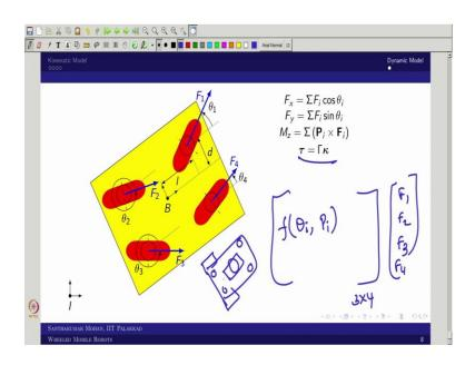
So, that is what I am trying to show here just for clarity you can see like I have taken  $\begin{bmatrix} F_1 \\ F_2 \\ F_3 \end{bmatrix}$ with respect to the  $\theta$  angles. So, now, this is what the sum that would be equal to  $F_x$ .
