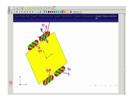
Now we will move to the fourth example where the mecanum wheel; so, now, the mecanum wheel is having what you call this is the hub axis and this is the roller axis, ok. So, I am putting this as a roller axis and this is the hub axis; so, now, where the force would generate?
