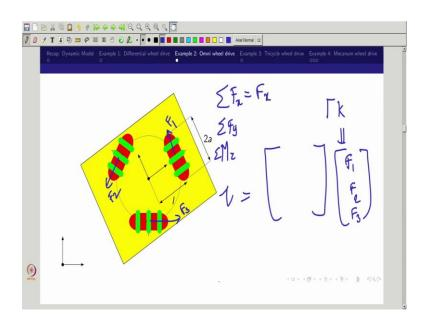
So similar way you can go with the further end where you can take a Omni directional wheel drive as the example. So, now what would be the direction of the you can say forward velocity? It would go like this. So, in the sense the same direction I am calling as a drive force which is  $F_1$  and this is the direction of velocity that would be  $F_2$  and this is
