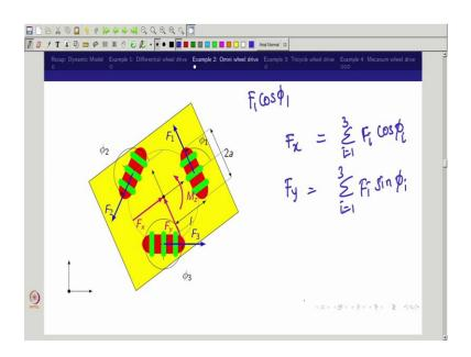
So, that is what I am actually like doing it, ok. So, now, what one can actually write? So, the F<sub>1</sub> x axis component would be. So, F<sub>1</sub>cos  $\phi_1$ ; so, I am rewriting as actually like F<sub>x</sub> is actually like written as. So,  $\sum_{i=1}^{3} F_i cos \phi_i$  right.
