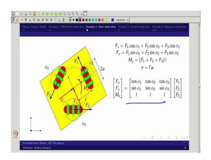
Because the passive roller in the y axis direction, that would not create any additional force input, that is why we are able to do this. So, that is what we are actually like done you see. So, now, this is what we are actually like going to use in the dynamic simulation later on.
