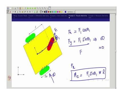
In the same way you try for a tricycle model where this is actually like a powered and as well as steerable wheel. So, then you can see that your force would be in this direction. So, this forced composition would be based on this  $\phi_1$  or  $\theta_1$  whatever you write  $\theta_1$  so,
