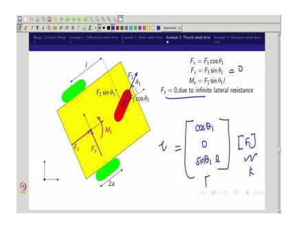
So, in the sense what would be your  $\gamma$  matrix? It straight forward right. So, what would be the  $\gamma$  matrix? So, since this is going to be 0. So, then this would be simply  $\begin{bmatrix} cos\theta_1 \\ 0 \\ sin\theta_1 l \end{bmatrix}$ . So, this would be simply F<sub>1</sub> right. So, this is what you can write as a T. So, this is what
