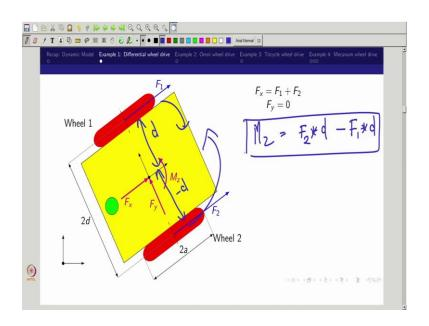
So, that is what we are trying to do. So, we see that this is the wheel force  $F_1$  and this wheel force  $F_2$ . So, now what would be  $F_x$ ? So, jut a sum of this right. So, that is what we are trying to write it right. So, what would be  $F_y$ ? In this case you see both are actually like a parallel force that too like along with what you call you can say along with the x axis of the you can say vehicle frame. So, then what you can see  $F_y$  would be 0 straight away right.
