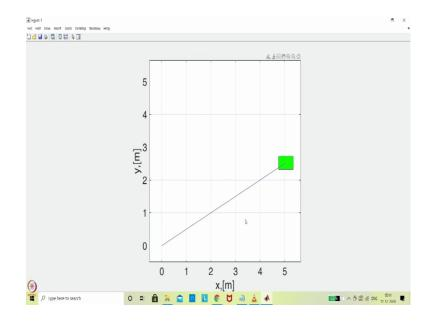
So, now, you can actually like see the animation. So, you can see like the 1 Newton force is acting on the body in the forward and 0.5 Newton is acting on the y direction. So, now, the vehicle is actually like moving both a longitudinal and lateral in the sense it is actually like moving in a inclined fashion.
