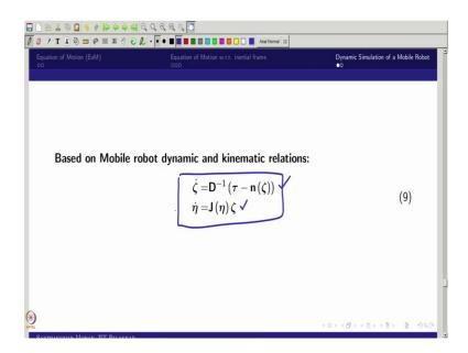
So, what we are trying to do. So, we are actually like trying to take one of the simplest equation which we have derived and this is the kinematic equation and this is the dynamic equation. I will be keeping the dynamic model as it is in the body frame because I told right my wheel forces or you can say my input forces would be with respect to body. So, I will keep it that.
