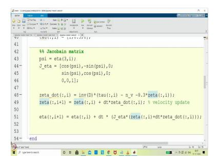
So, for example, I am assuming that it is a viscous friction. So, what that means? So, the viscous friction coefficient is known I assume that that is 0.3 and that is actually like in each and every state there is actually like the direct relations. So, in the sense  $\xi$  of actually like i. So, in the sense b v right when we write a second order system.
