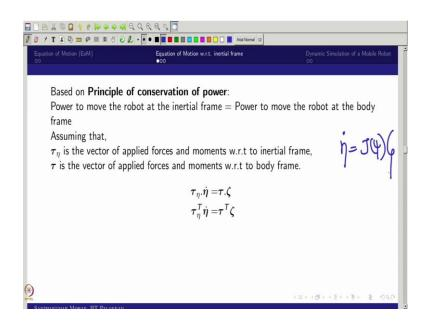
So, you can see like what we are doing that we are assuming that the  $T \times \eta$  is the vector of applied forces and moments with respect to inertial frame and tau is actually like vector of applied forces and moments with respect to body frame. I am actually like bringing this equation.
