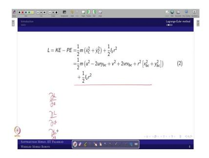
And we will actually like partially take the differentiation with respect to you call u then we will take v and take r and we will actually like try to take the time derivative that is what I am doing it one by one. First I write the bigger equation in the sense I expand this
