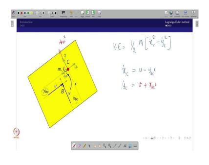
So, in the sense what one can see the body frame would have a linear velocities  $\begin{bmatrix} a \\ v \\ r \end{bmatrix}$  this
