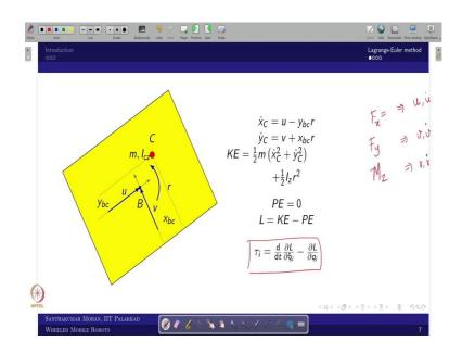
So, now, what you got it? The kinetic energy you got it now you substitute in a Lagrangian equation; what would be the Lagrangian equation? So, kinetic energy minus potential energy; so, this is the equation. So, in the sense the kinetic energy is the nothing but your Lagrangian and you take the Lagrangian Euler equation and you do it.
