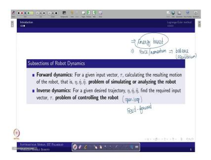
So, that is what I put it in this particular slide you can see forward dynamics means for a given input vector tau, calculating the resulting motion of the robot that is nothing but  $\eta$ ,  $\dot{\eta}$  and  $\ddot{\eta}$  whereas, the inverse dynamics is nothing but. So, for a given desired trajectory where  $\eta$ ,  $\dot{\eta}$  and  $\ddot{\eta}$  all desire and tried to find out what would be the input vector tau.
