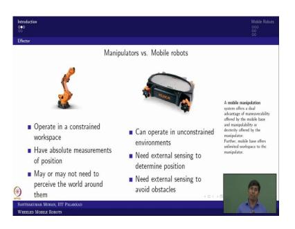
So, now we will move further. So, you have already classified the effector into two broad one is manipulator, the other one is mobile robot, we will talk more about you can say these in detail. So, what; that means, so the manipulator means it is manipulating the object around for example, I take my arm this arm is actually like manipulating the object around.
