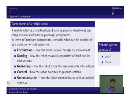
So, how these four pillars would be addressed. So, based on that you can actually see what are the components will come into a mobile robot. So; obviously, the mobile robot would be combination of both hardware and software, but here what we are interesting the components means the physical hardware.
