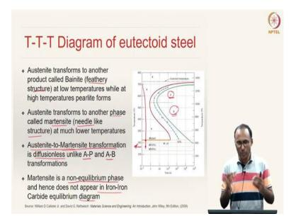
Austenite to martensite transformation is little different from austenite to pearlite or austenite to bainite transformation. The bainite microstructure is a feathery microstructure. If you look under microscope, when austenite transforms to bainite, you will see a feather like microstructure which happens at low temperatures, but at high temperatures, you will have pearlite.
