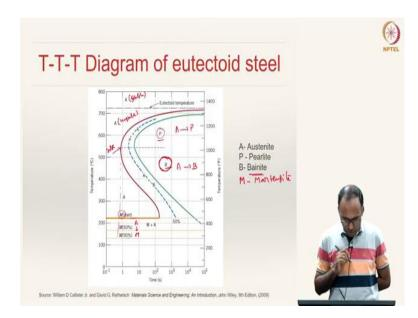
The complete TTT diagram over all the temperature ranges, below the eutectoid temperature is shown in this figure. This is the TTT diagram of eutectoid steel again. You can see that you have a transformation begin line and the transformation end line. And you have a temperature at which the transformation rate is maximum, and hence the time taken is minimum.
