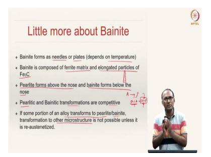
Bainite forms as needles or plates depending upon the temperature at which austenite transforms to bainite. Bainite is composed of ferrite matrix and elongated particles of cementite.
