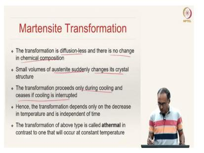
The transformation of martensite is diffusion less, and there is no change in chemical composition. Small volumes of austenite suddenly change their crystal structure because of the rapid cooling. The transformation proceeds only during cooling and ceases if cooling is interrupted; what is the meaning of that?
