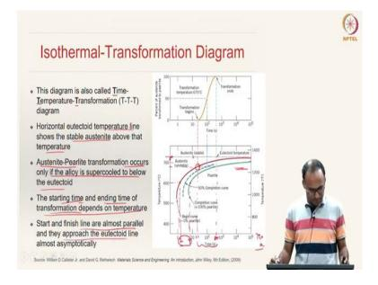
In the Time-Temperature-Transformation diagram or TTT diagram, here you can see this is the critical temperature, called as the eutectoid temperature above which austenite is stable below which actually austenite is not stable.
