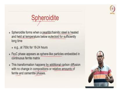
We will also look at something called spheroidite. Spheroidite forms when pearlite or bainitic steel is heated and held at temperatures below eutectoid for sufficiently long time. This is because, the cementite phase in this spheroidite microstructure looks like a sphere like particles embedded in continuous ferrite matrix; otherwise, the cementite network may be detrimental for the overall properties of the system.
