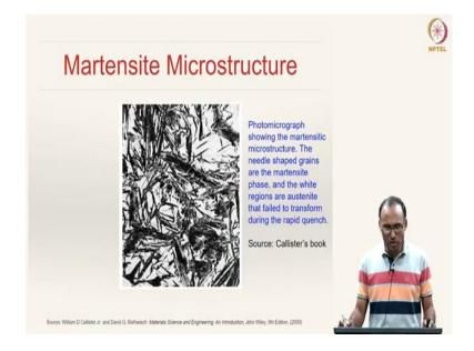
If you look at the microstructure of martensite under microscope, it looks something like this; which is as we have discussed – it is a needle like microstructure. The white regions here are the austenite that failed to transform during rapid quench. So, that is retained austenite and the black ones are your needle like structure called martensite.
