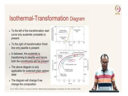
To the left of the transformation start line, austenite is unstable and to the right of the transformation end line, only pearlite is present. Pearlite is stable at this temperature. In between austenite starts transforming to pearlite - in some sense it is a two-phase region.
