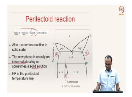
In this diagram, we will try to demonstrate the peritectoid reaction. So, peritectoid reaction is the one in which two solids, solid 1 and solid 2 upon cooling gives you solid 3.
