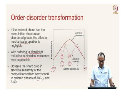
What is the implication of this ordered solid solutions to the properties of the alloys? If the ordered phase has the same lattice structure as the disordered phase, then the effect on mechanical properties is negligible. However, with ordering, a significant reduction in electrical resistance may be possible.
