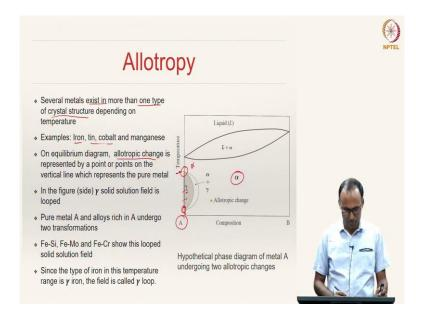
Several metals that we know of exist in more than one type of crystal structure depending on the temperature; at a lower temperature they exist in one kind of a crystal structure and if we increase the temperature, their crustal structure changes. Examples for such materials are iron, tin, cobalt and manganese.
