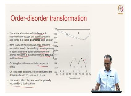
As we have already mentioned, solute atoms in a substitutional solid solution do not occupy any specific positions and hence that is called a disordered solid solution. If the random solid solutions are cooled slowly, then they undergo rearrangement of atoms, where the solute atoms move into definite positions in the lattice; that means, they are moving to a specific position, so as to give some order to the lattice structure. Such solutions are called ordered solid solutions.
