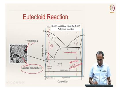
Alloy 1 which is in the liquid state to begin with, starts solidifying at this point, and then continuous to solidify. The solidification finishes here, and then the liquid would have transformed to  $\gamma$  - it is a single-phase region. So, here it is single-phase region, this is two-phase region, again this is single-phase region. It actually cools down in the single-phase region and again hits this line MN.
