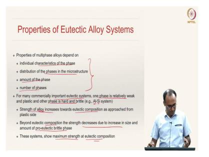
What are the properties of these eutectic alloy systems? The properties of multiphase alloys in general, depend on the individual characteristics of the phase, the distribution of the phases in the microstructure i.e., whether they are continuously distributed or not, the amount of the phase and the number of phases that are present. These factors are going to determine the mechanical properties or in general the properties of the alloy system.
