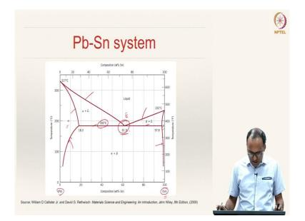
A real system that has such an alloy phase diagram that we have discussed so far -- three type of phase diagram is lead-tin system which is very well known to us as solder which is used for solder joints. So, here, lead is on the left-hand side, tin is on the right-hand side.
