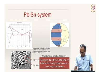
Why do alternate layers of  $\alpha$  and  $\beta$  form? The liquid here is having a certain composition and then, that is solidifying  $\alpha$ . The surrounding liquid becomes richer in  $\beta$  or richer in B and instead of forming B elsewhere, it is much easier for B to travel to the neighboring grains.
