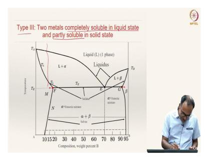
Welcome back. In the last class, we have looked at Type II alloys and we introduced a special reaction called eutectic reaction which happens when a liquid of a certain composition reaches the eutectic temperature. Thereafter, the liquid transforms into two new solids, and such a reaction is called eutectic reaction. We also discussed why eutectic reaction cannot be considered as a congruent solidification - it is incongruent in nature.
