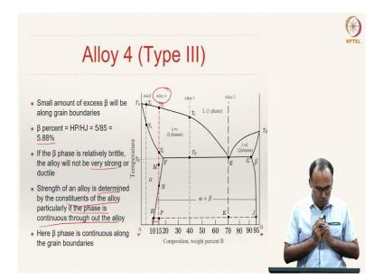
In the two-phase region, we can calculate the weight fraction of  $\beta$ . So, we can see that if you are drawing this line, the weight fraction of  $\beta$  will be,
