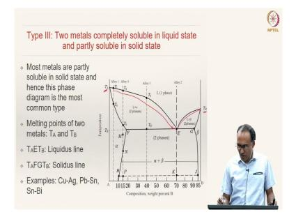
This is an important alloy system to look at because most metals are partly soluble in solid state. So, this is the most common type of phase diagrams. It can be seen here that  $T_A$  and  $T_B$  are the melting points of metals A and B.
