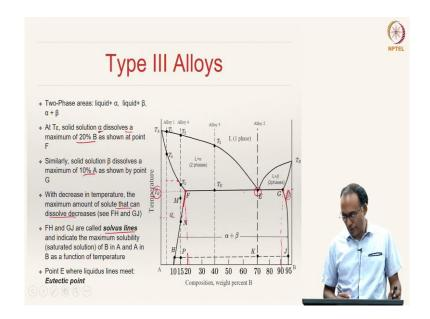
The two-phase areas as we have already discussed are liquid +  $\alpha$ , liquid +  $\beta$  and  $\alpha$  plus  $\beta$ . At temperature  $T_E$ , there is a maximum solubility for  $\alpha$ . The solid solution  $\alpha$  dissolves a maximum of 20% B; beyond that it cannot dissolve.
