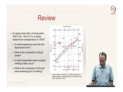
So, let us review once again. You have a copper-nickel alloy of composition 70 weight percent nickel and 30 weight percent copper. Where is 70 weight percent nickel - that is this point. It is slowly heated from a temperature of 1300° C. Initially it is at this temperature. From that temperature, it is slowly heated.
