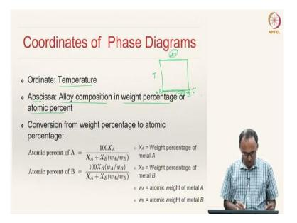
Before we actually start looking at phase diagrams, we need to see how these phase diagrams are drawn. Here, we have two variables, temperature and composition. Temperature and alloy composition are plotted on the y and x axes, respectively. The alloy composition can be written either in weight percentage or atom percentage. We already know how to convert from weight percentage to atom percentage, and vice-versa.
