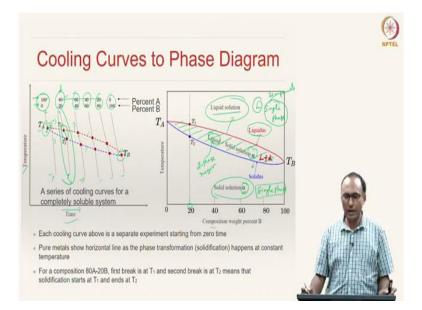
In this course, we will start trying to understand phase diagrams from cooling curves right away. On the left-hand side in this graph, you have temperature as a function of time. Here, the top line represents weight fraction of A, and bottom line represents weight fraction of B. When the pure metal A, i.e., 100% A is cooled from a very high temperature which is in liquid state, it reaches its solidification temperature  $T_A$ . Let us say metal A has higher melting point than metal B.
