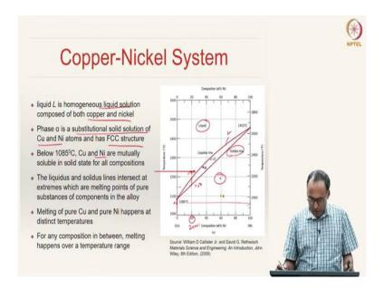
Here, we are showing the phase diagram of copper-nickel system. Copper is a low melting alloy and nickel is a high melting alloy. Previously we have seen the phase diagram this way; instead of plotting the low melting point alloy on the right-hand side, if you plot it on left-hand side, this is how it looks like.
