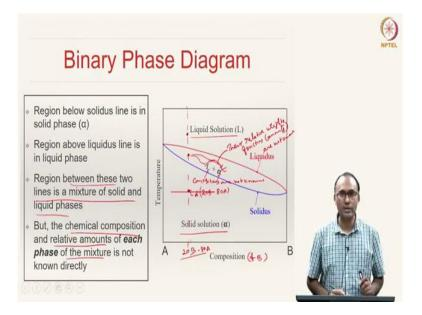
So, here I am summarizing -- the region below the solidus line is called solid phase, the region above the liquidus line is called liquid phase, and the region between these two lines is a two-phase region, a mixture of liquid solution and a solid solution alpha.
