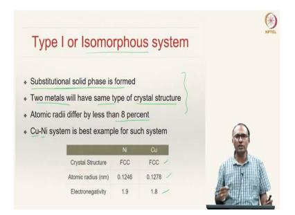
Now, we will look at Type I or isomorphous alloys. Isomorphous alloys are the ones which have complete solubility in solid state as well as liquid state. As we have looked at the Hume Rothery's rules, 100% solubility is possible only when the atoms are of similar sizes.
