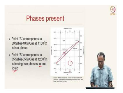
For instance, in this phase diagram, you see the point A which corresponds to 60% nickel, 40% copper at 1100° C, and is in  $\alpha$ -phase -- it is a single-phase region. However, point B here, corresponds to about 35% nickel, 65% copper at 1250° C, but having two phases - alpha and liquid solution.
