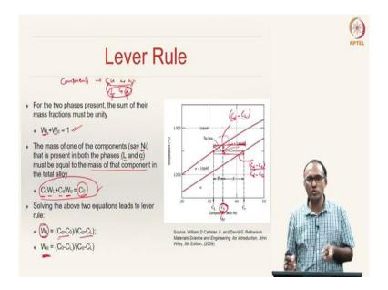
We know the compositions, but how do we find out the fraction of liquid that is present, what is the fraction of the solid that is present? For that, we use something called lever rule. So, what is that lever rule?
