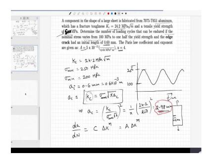
A component in the shape of a large sheet is fabricated from aluminum which has a fracture toughness of 24.2 MPa $\sqrt{m}$ , and a tensile yield strength of 500 MPa. Determine the number of loading cycles that can be endured if the nominal stress varies from 100 MPa to one half of the yield strength.
