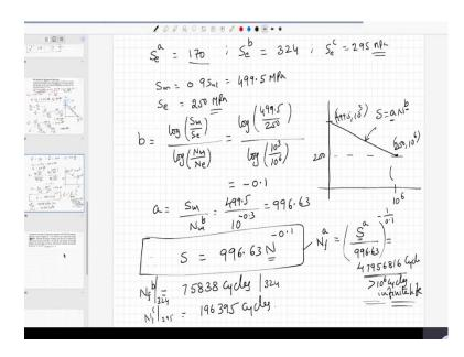
$S_{ut} = 555$  MPa,  $\sigma_a = 277.5$  MPa, that is half way somewhere here and let us say this is the failure point. Then, you need to join these lines and then this corresponds to a particular number of cycles  $N_f^a$ . Similarly, if  $\sigma_m = 200$  MPa, that is somewhere here,  $\sigma_a$  is here that is let us say point b 207.8 MPa, then that would be the corresponding failure line.
