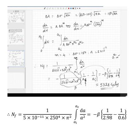
You can calculate the value of  $\beta$  and then you find out  $N_f = 5328$  cycles; that means, even if you have an initial crack of length 0.6 mm, you will still be able to retain the functionality until the cycle number of cycles are about 5328; until then the specimen will be safe.
