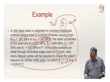
This is a simple example problem, wherein you have a mild steel plate which is subjected to constant amplitude uniaxial fatigue load to produce stresses varying from  $\sigma_{\text{max}} = 180 \text{ MPa}$ ,  $\sigma_{\text{min}} = -40 \text{ MPa}$ . Please pay attention here, as  $\sigma_{\text{min}}$  is negative.
