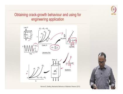
How do we go about using this in the real-life design? You do a laboratory test on a specimen of the kind of loading that you would expect in the real-life scenario on a laboratory specimen and then, do this for different  $\Delta P'$ s.  $\Delta P = P_{\text{max}} - P_{\text{min}}$  as you have seen here.
