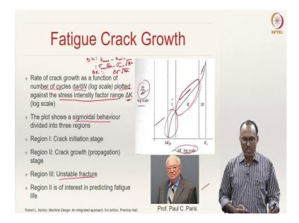
The rate of crack growth as a function of number of cycles denoted by  $\frac{da}{dN}$ , plotted against the stress intensity factor range  $\Delta K = K_{\text{max}} - K_{\text{min}}$ .
