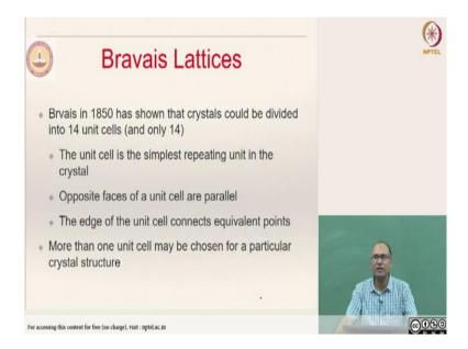
Similarly, for any unit cell you can define the levels of symmetry that is possible. And usually, the geometries of the unit cells are defined based on the symmetry level.
