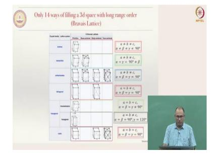
These are the 14 ways of filling a 3D space, these are the 14 possible Bravais lattices. So, you have cubic primitive unit cell and there is something called body-centered cube and face-centered cube. We are familiar with these two things, right? Body-centered cubic and face-centered cubic structure, we have looked at in your previous class.
