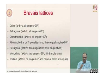
And these are basic seven geometries of the unit cell that are possible. Cubic means *a* equal to *b* equal to *c*, all angles  $\alpha$ ,  $\beta$ , and  $\gamma$  are equal to 90 degrees. In Tetragonal, two sides are same (*a=b*). If you take a cube and pull it, then it becomes tetragonal. That can also be a possible unit cell. If you pull in this direction and pull in this direction such that
