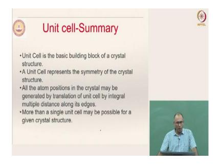
The summary of unit cells is a basic building block of a symmetry structure, it represents the symmetry level of the crystal structure that we are looking at. All the atom positions in the crystal may be generated by translation of unit cell by integral multiple distances along its edges called lattice vectors. More than a single unit cell may be possible for a given crystal structure. That is what we have learnt about unit cells.
