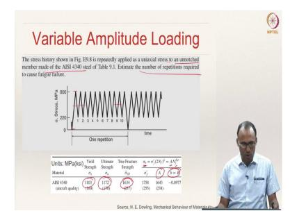
You can now solve this problem. The stress history shown is repeatedly applied as a uniaxial stress to an un-notched member of AISI 4340 steel. Estimate the number of repetitions required to cause fatigue failure. So, this is one stress amplitude, and this one is another one.
