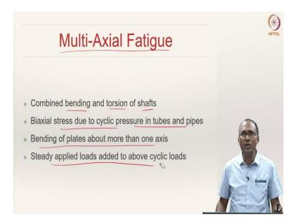
When you have multi-axial loading, you need to consider all the six stress components. Hence, we need to see how one would actually study the failure when the component is subjected to a multi-axial loading and that is what we designate as Multi-Axial Fatigue.
