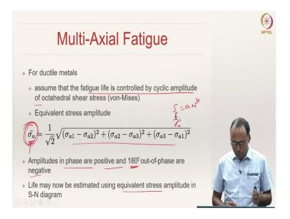
Here, we are going to prescribe a methodology to deal with multi-axial fatigue, wherein the direction of the principal stress remains constant, however, the other stress components are changing or fluctuating.
