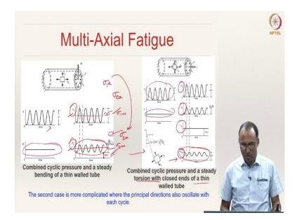
This is one example of a combined cyclic pressure and steady bending of a thin-walled tube. This is cyclic pressure and steady bending, i.e., bending moment is constant. As a result, you will have cyclic pressure loading. A steady bending load should be added to that, and as a result, the resultant system is subjected to such a variation.
