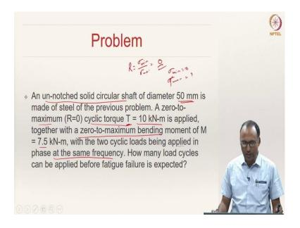
Here, we have a problem wherein an un-notched solid circular shaft of diameter 50 mm is made of steel. This is same as the previous problem. A zero-to-maximum cyclic torque, so that means,  $\sigma_{min} = 0$ ,  $\sigma_{max} = \tau_{max}$ . Here we have torque, torque means you are cycling shear stresses.
