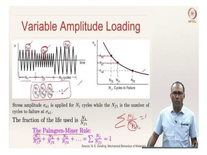
So, until now, the kind of problems that we have dealt with are having the same stress amplitude, i.e., the stress amplitude is uniform. However, in real systems, you may also have variable amplitude; that means, during this loading, the stress amplitude might change as shown in this figure here.
