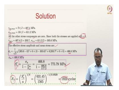
So, you calculate  $\tau_{xy,max} = 407.4$  MPa because minimum is 0. We are only calculating the maximum values now, and this is from bending. All the other components are 0, because these are the only two things that are acting. Both the stresses are applied such that the stress ratio R = 0.
