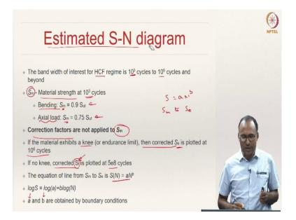
We have looked at five correction factors: load factor, size factor, surface factor, temperature factor and reliability factor. After calculating these five correction factors, you need to correct your endurance strength by using the formula,
