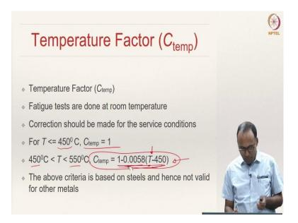
The next factor is the temperature factor, denoted by  $C_{\text{temp}}$ . Usually, the rotating beam bending tests are done at room temperature, and hence correction should be made for service conditions. We are following these procedures for steels, but for other materials, similar expressions should be available. For  $T \leq 450^{\circ}$  C,  $C_{\text{temp}}=1$ , i.e., it need not be changed.
