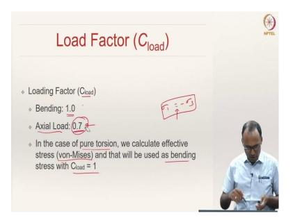
Let us go by each and every factor. The first factor that we are going to focus on is something called load factor, denoted by  $C_{load}$ . You know that the rotating beam bending test data is obtained by applying a bending load. If your real-world application is also subjected to the bending load, then you use load factor to be 1. But if the real-world application is using axial load factor, then you should use a load factor of 0.7.
