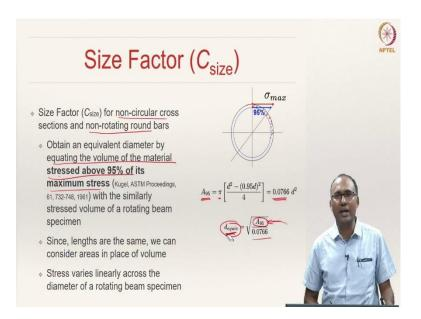
I will explain briefly how one should deal with non-circular cross-sections and also nonrotating round bars. If it is not rotating also, it is important because if it is not rotating then the material point that is under high stress region probably continues to be in high stress region and so on. So, it is also important to see what happens for the non-rotating bar and non-circular cross-sections.
