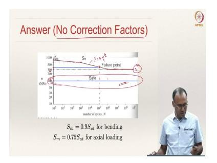
Without applying any correction factors this is exactly the same problem. For 100 MPa stress amplitude, that specimen turned out to be perfectly safe, right? However, after applying the correction factors, you have clearly seen that the material is not safe anymore even at 100 MPa stress amplitude.
