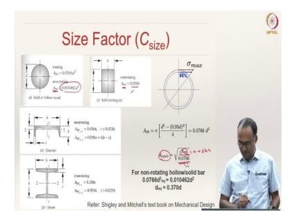
Let us see one quick example. For a rectangular cross-section, you know that  $A_{95} = 0.05bh$ . That is the area subjected to greater than 95 percent of the maximum stress. All that you need to do is, in order to calculate the equivalent stress, you plug in  $A_{95} = 0.05bh$ , and then calculate the equivalent diameter.
