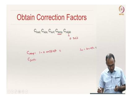
So, we can right away write  $C_{reliab} = 0.753$ . Since the working temperature is 500° C,
