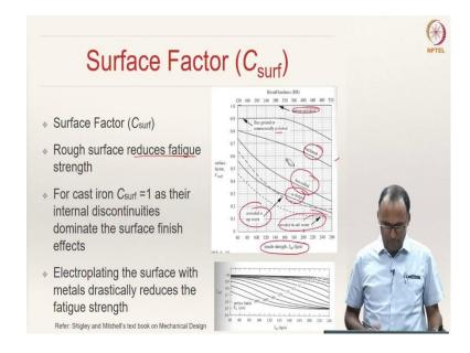
That is about size factor. Until now, we have looked at the load factor and size factor, and now let us discuss about the surface factor. The surface finish of a material is going to significantly influence the fatigue strength of the material. The rough surfaces reduce the fatigue strength, and smooth surfaces increase (correction: do not affect) the fatigue strength. Hence, you need to account for the surface finish.
