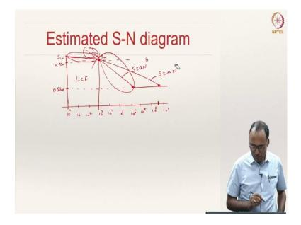
So, how do we do that? Let us say this is  $S_{ut}$ , this is  $0.9S_{ut}$ , and this is my  $0.5 S_{ut}$ . As we have discussed, the HCF regime is from  $10^3$  cycles. That is the point  $S_m$  and  $S_e$  is here, and that is the straight line  $S = aN^b$ . The first point is here.
