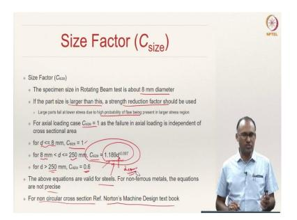
The next factor is the size factor, denoted by  $C_{size}$ . The reason why we have to include this size factor is because the rotating beam bending test uses a cylindrical specimen size of 8 mm diameter. However, the real-life scenario uses different sizes of the components, right? The component size need not be 8 mm all the time.
