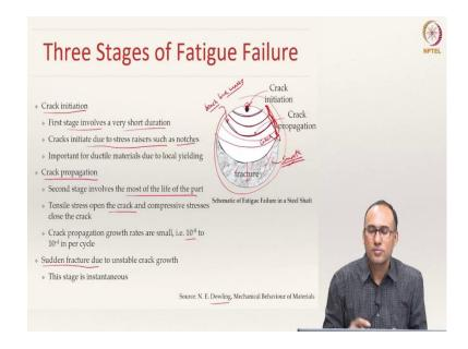
Let us now look at another important aspect in understanding the mechanism of fatigue failure. How does a component fail, when it is under fatigue loading? The fatigue failure in general can be classified into three stages.
