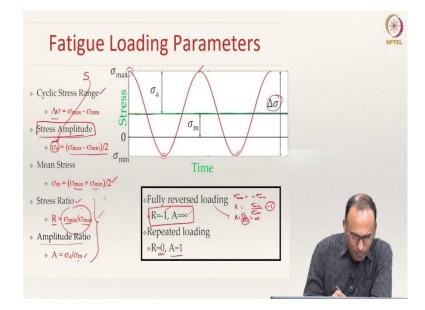
Before we move on, this is a very important slide where we need to understand the definition of various parameters when we are talking about fatigue loading. Here we are showing a fluctuating loading scenario. This is the most general loading scenario, wherein you have a minimum stress to be negative, you can see this is 0 and maximum stress to be positive.
