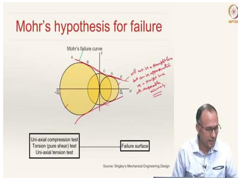
The left most circle is uniaxial compression, the right most yellow circle is uniaxial tension and the middle circle is basically a pure shear case, right? Then you can draw a common tangent to all these three circles. This common tangent represents the failure surface. This was proposed by Mohr and hence this is what is called Mohr's failure theory for brittle materials.
