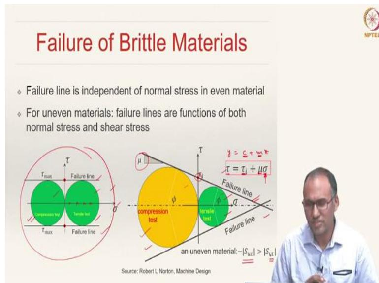
Let us now see how the failure surface looks like. We have discussed about the 2 kinds of materials in the last class, i.e., even and odd materials. What do we mean by an even material? An even material has both the tensile and compressive strengths to be equal in magnitude.
