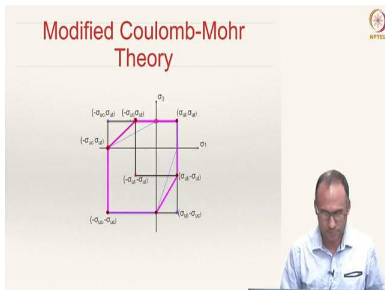
People later actually looked at the experimental data and they have modified the failure theory a little bit, called this as modified Mohr-Coulomb theory wherein, instead of connecting this line and this point, you actually connect the  $\sigma_{ut}$  and this is what we call modified Mohr-Coulomb theory. This has actually been modified from the Mohr-Coulomb theory by looking at the experimental data.
