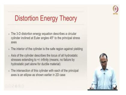
How does the distortion energy theory equation look in a 3-dimensional space where your axes are  $\sigma_1$ ,  $\sigma_2$  and  $\sigma_3$ ? The 3D distortion energy equation describes a circular cylinder inclined at Euler angles 45° to the principal stress axis, and interior of that cylinder is safe region against yielding.
