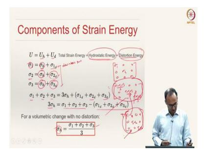
The total strain energy that is stored in a material can now be decomposed into two parts; the hydrostatic energy and the distortion energy. The hydrostatic energy  $U_h$  is responsible for size change or volume change, and the distortion energy  $U_d$  is responsible for shape change.
