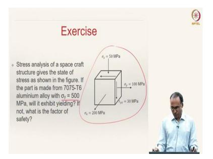
Let us do this problem by applying distortion energy theory and try to understand. So, the stress analysis of a spacecraft structure gives the state of stress as shown in this figure. If the part is made from an aluminum alloy, whose yield strength is 500 MPa. The question is, will this stress state cause the material to yield? If not, what is the factor of safety? It is extremely important to write  $\sigma_x$ ,  $\sigma_y$  and  $\tau_{xy}$  with proper signs.
