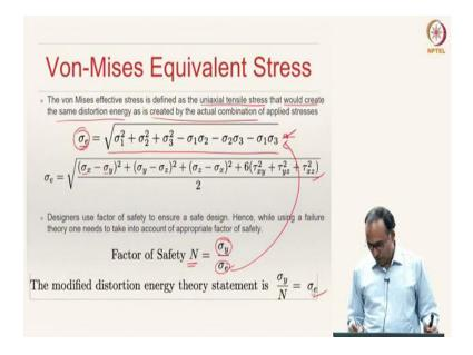
The distortion energy theory states that, this stress which is a complex equation taking into account the elements of the principal stress tensor -- this value is compared with a scalar which is  $\sigma_v$ .
