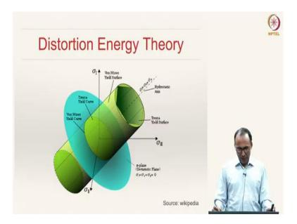
Ignore the hexagonal shape that is shown there, and focus on the circular cylinder; you see that this is the axis. Here you have  $\sigma_1$ ,  $\sigma_2$  and  $\sigma_3$  and the cylinder is inclined at a 45° angle with all the principal axes.
