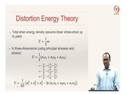
The total strain energy density for a one-dimensional case assuming linear stress-strain relation up to yielding is
