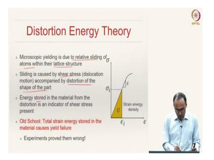
We will now start discussing about the distortion energy theory. The microscopic yielding that we have discussed in the mechanical behavior module is due to relative sliding of atoms within the lattice structure, right? The sliding is caused by shear stress or in other words the plastic deformation is caused by dislocation motion, which is accompanied by the distortion of the shape of the part.
