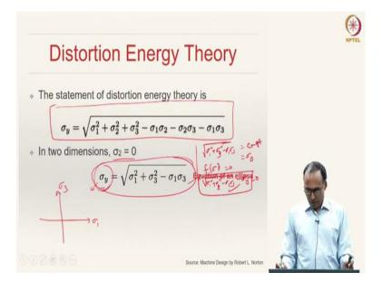
The mathematical statement of distortion energy theory is this, which basically represents the boundary of the failure surface. In 2D, for a plane stress case,  $\sigma_2 = 0$ ,
