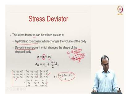
Let us now look at the deviatoric part of the stress tensor, that is also called stress deviator. So, the stress tensor  $\sigma_{ij}$  can be written as a sum of hydrostatic component and deviatoric component.
