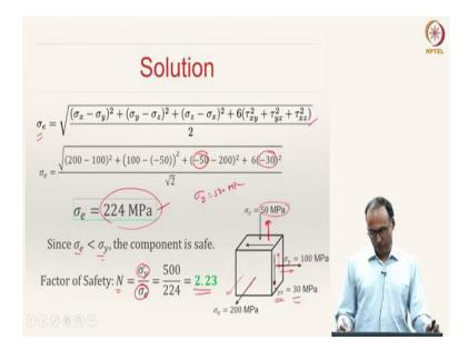
This is our equivalent stress. It is good to write in the x, y, z frame of reference rather than writing in the principal frame of reference; here we are given x, y, z data and not the principal data, because you have a shear stress component here. So, that is not a principal state of stress.
