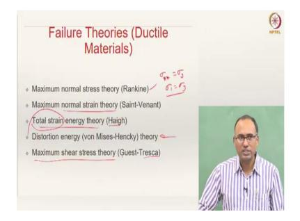
There are different failure theories as we have discussed. Maximum normal stress theory, also called Rankine theory is named after Rankine who prescribed this theory. This theory states that when the maximum normal stress is equal to yield strength of the material, that is when the material fails.
