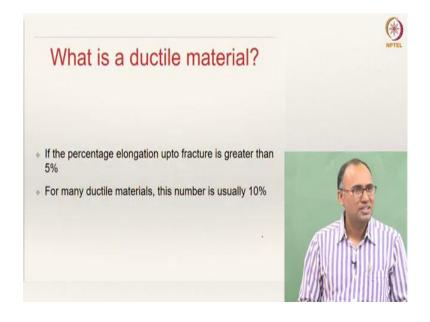
How do you consider a material to be ductile material? What is the limit? Can you say in black and white that this is a ductile material and this is a brittle material? Are there no materials which are somewhere in between? It is always possible, right? Hence, you need to have some quantification to classify a given material as a ductile material or a brittle material. So, the classification is basically percentage elongation.
