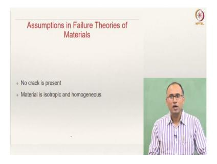
As far as this class is concerned, we have certain assumptions when we are defining failure theories. The first assumption as far as static failure theories are concerned is that there are no cracks present in the material; it is a very important assumption. The moment there is a crack, then you may have other issues. Another important assumption is the material is isotropic and homogeneous.
