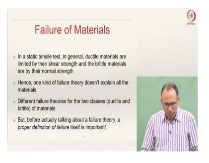
In a static tensile test, in general, ductile materials are limited by their shear strength and brittle materials are limited by their normal strength, because they fracture by normal strength.
