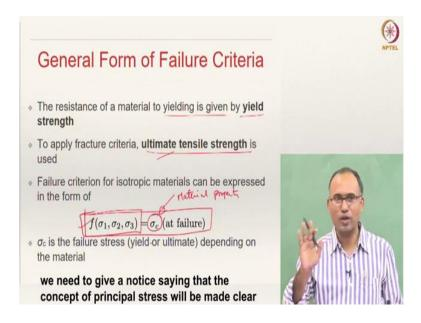
How does the general form of failure theory look like? What should be the functional form ok? Let us say the resistance of a material to yielding is called yield strength; that is something that we know, and that is for ductile materials.
