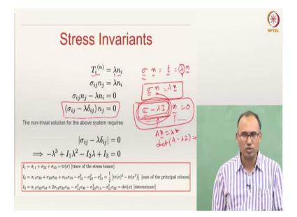
I can describe my traction direction to be same as the direction of the normal right. I can write this  $\lambda$  is a scalar.
