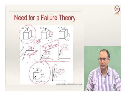
Now, we need to establish the need for failure theory. Why do we need to come up with a failure theory? So, here you have 3 scenarios. You see the first case. Here, we are considering a material which is elastic perfectly-plastic.
