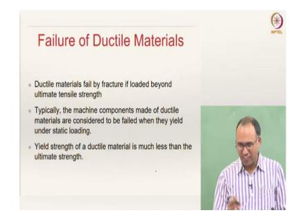
As we have already mentioned several times, ductile materials fail by fracture if loaded beyond ultimate tensile strength; until then they would not fail by fracture. But, when we are designing, we will not go up to there; we consider them to be failed when they yield under static loading. For ductile materials, it is important because the yield strength and ultimate strength are not the same.
