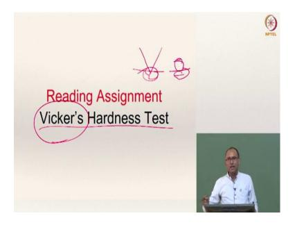
The indenter is different in Vicker's hardness test and the way the Vicker's hardness test works is similar to Brinell hardness test. It also reports the load by area unlike Rockwell hardness
