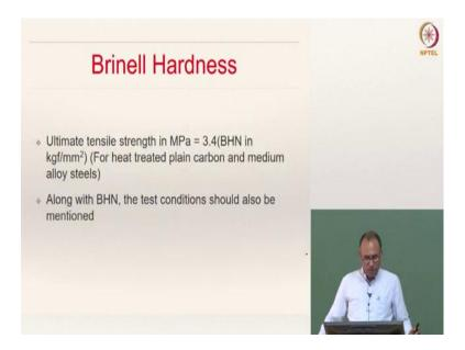
By measuring the Brinell hardness, you can also sort of estimate the tensile strength of the material; it is only an empirical formula suitable only for plain carbon and medium alloy steels. That means, if you know your Brinell hardness number in  $kgf/mm^2$  from the previous formula, if you multiply that with the 3.4, the number that you get is approximately equal to the ultimate strength of the steel in MPa.
