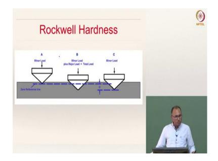
So, this is how you will apply you apply a minor load and then a major load and measure the depth of indentation. That depth of indentation is shown on the dial.
