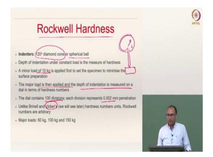
If you change the indenter from steel ball to some other indenter shape and if that indenter shape happens to be a 120 degrees diamond cone (or sometimes spherical ball), then, you will have something called Rockwell hardness indentation. As above, you apply a constant load and measure the depth of indentation.
