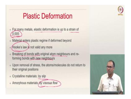
Let us move on to plastic deformation. As you load the specimen beyond elastic limits, the material gets into plastic regime. This means that you are activating the dislocation motion and thus the material plastically deforms. So, for many metals, the elastic deformation is only up to a strain of 0.005 beyond which it enters into the plastic regime. Note that this is only a thumb rule.
