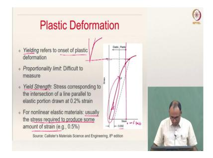
In the previous lecture, we saw the initial portion of the graph. Let us now look at the next portion. This region (marked) is the plastic deformation. Yielding refers to the onset of plastic deformation, i.e. the point at which your plastic deformation starts. This point is referred to as the yield point.
