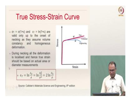
The first 2 expressions are valid only till the onset of necking as they assume volume constancy and homogenous deformation. So, similarly, you can also write a relation between true strain and the engineering strain.
