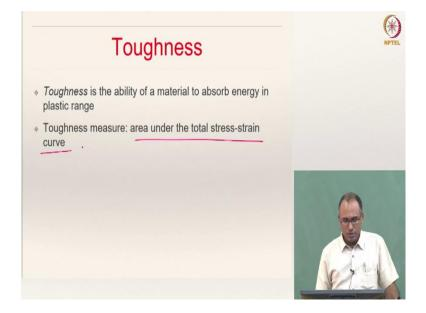
Toughness is the ability of a material to absorb energy in the plastic range. It is the area under the total stress strain curve.
