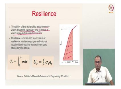
Resilience is defined as the ability of the material to absorb energy when deformed elastically and to return it when unloaded. This is an important property to consider in the design of springs, for instance.
