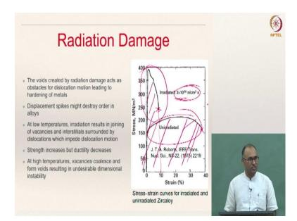
This is the stress-strain graph for zirconium alloy Zircaloy. This is an irradiated sample and this is an unirradiated sample. So, this is the dosage and you can clearly see that the material has become extremely brittle. After this much of irradiation, the material has become extremely brittle.
