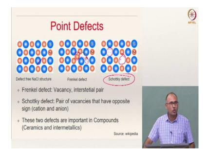
For instance, this is NaCl structure which is defect free, and here you have a Frenkel defect. Frenkel defect means an interstitial and a vacancy side by side. If you have a vacancy here and you do not have an interstitial here, but far away, then those two cannot be called as Frenkel pair because they should be close to each other. And there is another kind of defect which is called Schottky defect.
