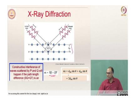
$n\lambda = \overline{SQ} + \overline{QT}$  $n\lambda = d_{hkl} \sin \theta + d_{hkl} \sin \theta$  $n\lambda = 2d_{hkl} \sin \theta$
