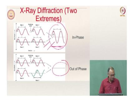
This picture gives you a little bit more information. So, when you have 2 waves: wave 1 and wave 2 which are in phase, their interference causes some amplification and you get a
