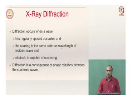
We can use diffraction of light or here X-ray diffraction and we know how diffraction occurs, right? Diffraction occurs when the wave hits regularly spaced obstacles. If the spacing is the same order as the wavelength of the incident wave and when the light is hitting, if the obstacle is capable of scattering the light only then you will have the diffraction.
