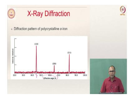
Alright. So, I will skip this, and then this is how a diffraction pattern looks like when we do the X-ray diffraction for a given powder sample. So, this is the X-ray diffraction pattern of the polycrystalline  $\alpha$ -iron. By knowing at which diffraction angle you have peaks, you will be able to figure out which material you are looking at.
