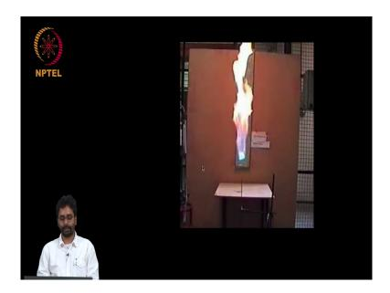
Now, you see that the tip is becoming unstable, the you know the flame has lifted off and become turbulent; now, more or less the entire length of the flame is turbulent now. The base is bluish and it is because, it is lifted off there is some pre mixing that is happening till the point of ignition and the flame stabilizes at a point where the turbulent flame speed is matched by the local velocity.
