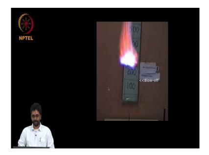
Now, we will also see blow off of this flame. I will play it one more time, yeah it is already playing (Refer Time: 01:57). You must have seen that it is the tip that becomes turbulent first and then the disturbances propagate to the base, and when the disturbance propagates to the base flame lifts off and you have lifted flame for a range of Reynolds numbers and then it close off.
