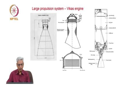
The flow to the combustion chamber is specific streams, it is true even here, they take a specific track and come here; which means, if you take a group of injectors you can track them, they actually move with the same O by F.
