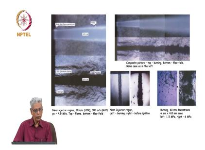
More pictures here, you will see the flame from that from the actual combustion system; LOX jet and bright spot which is a recirculation zone close to the injector phase are different phase and well what else can we get out of that. The same picture, top is burning, bottom is the actual flow field in the system; when it is not burning, you can look at how things are ok, here the jet flow, but actually combustion system is not what you see.
