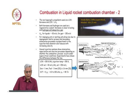
Non hypergolic propellants lox kerosene, lox hydrogen; both kerosene and hydrogen are used as a regenerative coolants. Kerosene is close to the boiling point and hydrogen will always be a gas. V inject V injector velocity of the injector a for liquids is 30 meters per second, gas around 150 meters per second; and density is low in spite of the fact at high pressure. And so, you need a cross section which is large; even if you provide further, the velocity has to be on this class.
