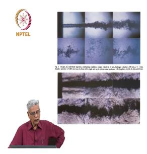
From the LOX jet core, thread like structures develop and grow. They do not detach, but dissolve and fade away Several tens of diameters downstream LOX core breaks up into large LOX lumps dissolving the same way.
