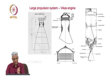
I just want to show you the large propulsion system called it Vikas engine, which is actually being deployed in ISRO. It is the interesting combustion system, you have oxidizer fuel coming in; you have six injectors as you will see here, impinging injectors, radially they are coming into the combustion chamber, combustion occurs here.
