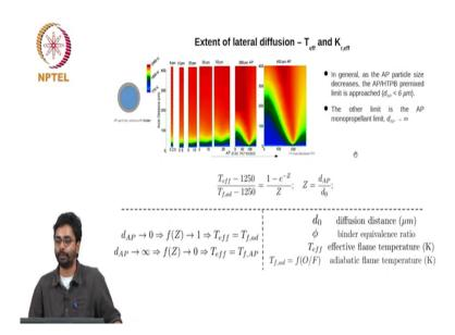
So, far we have been looking at either pure AP or homogenous AP HTPB mixtures, but in reality we have large AP particles surrounded by binder ok. Calculations were done by Gross and Beckstead for such a configuration with AP particles of various sizes surrounded by binder matrix such that the total solid loading of AP is 86 percent. They maintain the same solid loading and that calculations for various sizes of AP particles ok.
