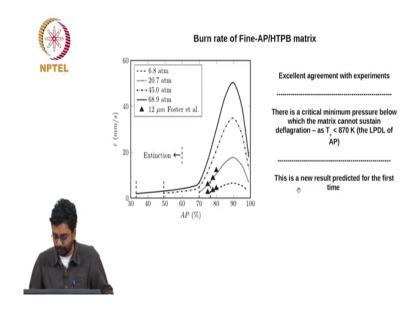
But before that how do we know that this parameter set is good enough? So, using this parameter set calculations were made for homogenous compositions of you know variety of compositions with AP fraction ranging from as low as 30 percent to as high as 95 98 percent. Some limited experimental data was available and the productions and the comparisons were in reasonable agreement.
