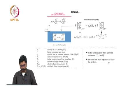
So, now we have one equation and in the surface heat balance equation there are three unknowns, the surface temperature is unknown, the burn rate is unknown and the other thing that is not known is the flame stand of distance ok.
