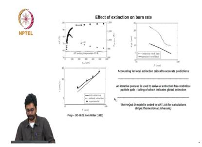
So, I said that there is no hard data available for validating the extinction limits for homogeneous compositions, but what we found evidence in by other means this is prediction for a particular composition taken from Miller 1982. When we do not account for extinction the predictions is shown by this dotted line and the data are the triangles which are actually the error bars are about 10 percent. So, the deviation and burn rate is quite significant it is about 20 percent.
