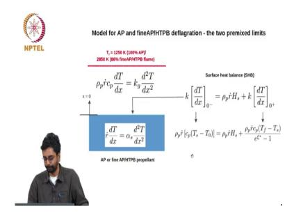
Now, we can solve for these slopes by integrating the convection diffusion, one dimensional convection diffusion in the solid phase. I am sorry one dimensional convection diffusion in the gas phase and the heat conduction equation in the solid phase and these have simple solutions.
