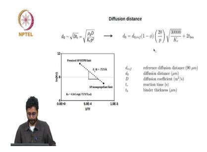
We already discussed this in some detail. The extent of lateral diffusion is proportional to square root Dt r this we have already discussed; t r is the reaction time which is density divided by the reaction rate that is exactly what is done here. Density is rho g divided by reaction rate which is K r p squared diffusion constant ok. This idea you can express in a slightly simpler form as shown here.
