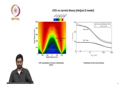
So, let us look at the predictions in the theory. So, as I said that at the limits we definitely know that the relationship works, but this is to show that at intermediate sizes also we get the correct results. The thick lines the continuous lines are the predictions from CFD by Gross and Beckstead, the dotted lines are the predictions of the current model they are in they are in very good match ok. In fact, this is what was used to validate the lateral diffusion model.
