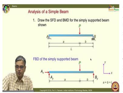
view more than the sign of the bending moment you are worried about the magnitude of the bending moment that is very important. The magnitude is very important for your design purpose that is what you are really looking at. Nevertheless, when I want to draw the diagram along the length of the beam, I
