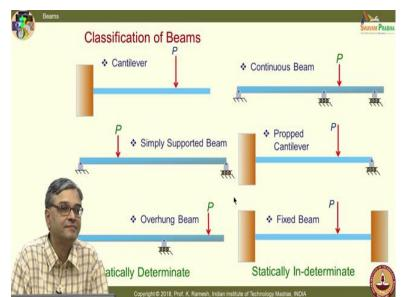
support and I have a slender member like this, I have an end load and this has a particular name this is called a cantilever.
