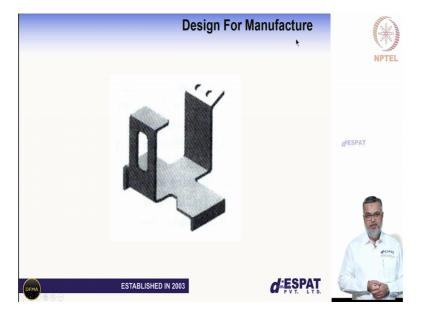
The other module that we have in you know software is called the design for manufacturing module so in order to explain that I have taken a simple example of sheet metal component here.
