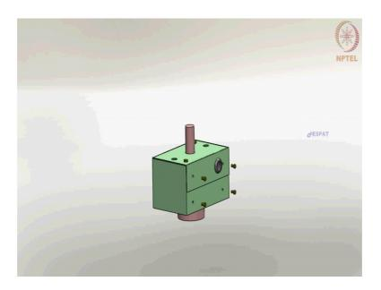
So, you see that the base is a first part that is going to be assembled followed by a sequence of components the one that look like a cylindrical component is a motor that is supplied by vendor. And let us assume the rest of the parts are made in house where for this product to be fabricated.
