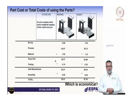
So, if you do a scientific analysis of these two parts using the design for manufacturing method. You will be surprised to see that at one aspect we were probably right. Which is the cost of material in the one that is marked is wrong being higher, but it wins out and the other attributes that contribute to the cost of manufacturing the part which is in terms of the setup the process in one tool you could probably stamp the part.
