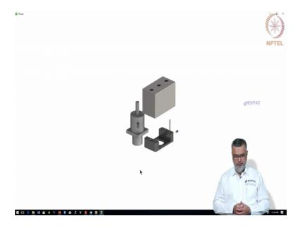
Where in the cover and then and plate is ones envelop part and instead of having those separate 6 or 8 fasteners. We have one envelope shape which could be which could be used to cover this whole motor assembly.
