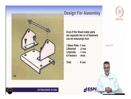
It is quite evident that if you were to integrate the threading as a part of the base you would probably be able to save so, many of these fasteners components. So, 24 part product would probably be 8 part candidate.
