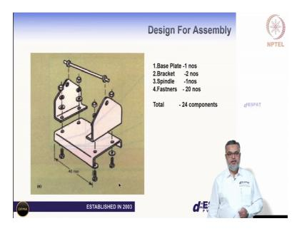
That is a DFMA has two module that look at this aspect of a product design the first of which is called the design for assembly. The design for assembly for software has two module one is called the design for assembly module and the other one is called the design for manufacture.
