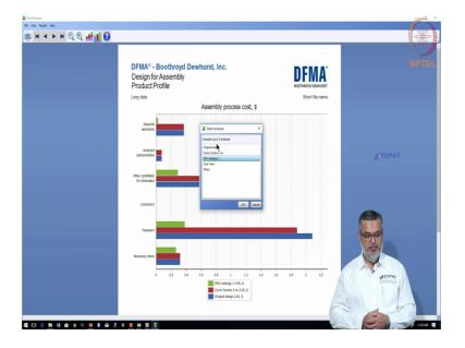
Then interesting attribute that you will probably come out and this attribute is very evident in most product builds which is the fastness as you can see here is taking about close to 160 seconds of assembly time out of a total of 260 seconds of the products assembly.
