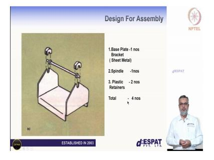
Little more improvised design would probably look something like this have a single part which going to probably a sheet metal or plastic component. And hold that spindle in position by means of plastic or metal or rubber retainers 4 part candidator.
