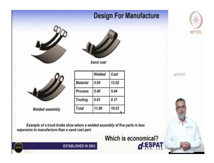
Let us look at one more example of published case study for one of our customers. If you would see most of the automotive world uses casting as the process for manufacturing brake shoes and the in the process of looking at newer ways of manufacturing our we have explode; let us say a make manufacturing the same part through sheet metal.
