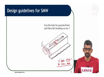
There is a food for thought; there are 2 operations in a sheet metal to come to this component. So, one is bending here and the other one is the hole.
