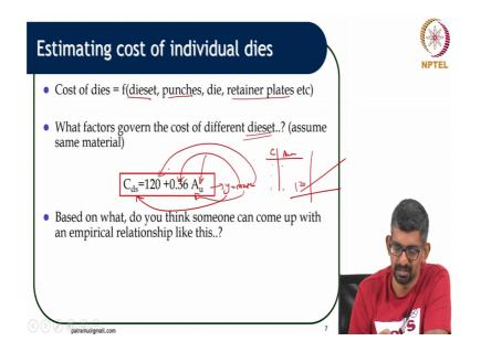
Similar to the other one we are interested in estimating the cost ok. So, in this particular case; obviously, the die cost itself is also included and how do you go about it? So, the cost of the die is the die set, the male and the female part, the punches, the retainer plates. What factors govern the cost of the different die set?
