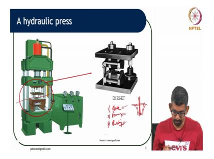
So, this is a hydraulic press, sometimes it is also these are called your die set or your press tools, right. So, usually the press tool has 3 elements at the top and 3 elements at the bottom. There are different process that a particular component goes through before it
