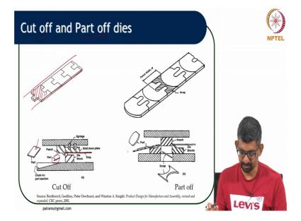
So, there are a couple of things in terms of the dies depending on the finished product that we get or the finished component that we get they can be classified as a cut off part cut off or part of dies. What is the cut off? Take such a design there will be no scrap per say ok.
