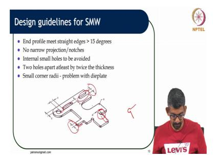
So, this is some design guidelines for sheet metal working. So, the point is the end profile meet straight edges only at greater than 15 degrees. So, the other one is there is no narrow projection or notches. So, you cannot have very narrow notches or projections that are very narrow.
