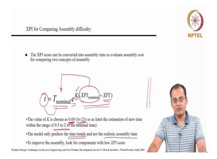
So, we can do an assembly operation and find the time and benchmark that and use that as the standard time. We compute the assembly difficulty for this method, that is XPI indicator and we take these two as the numbers and do a mapping; that means, if there is a change in the assembly score, how far the assembly time can change. So, this is again
