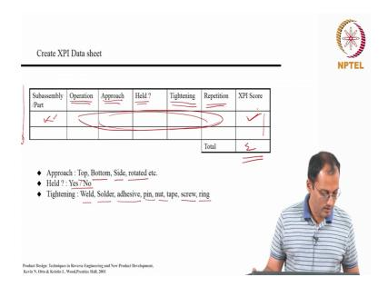
So, the XPI data sheet looks like this. So, we annotate the parts or the sub assemblies the corresponding to each part, we would like to describe the assembly operation. The approach direction, whether the part needs to be held when the assembly is being carried out and what kind of tightening or you know, the operation, fixing operation that needs to be employed and how many times, we are repeating that operation.
