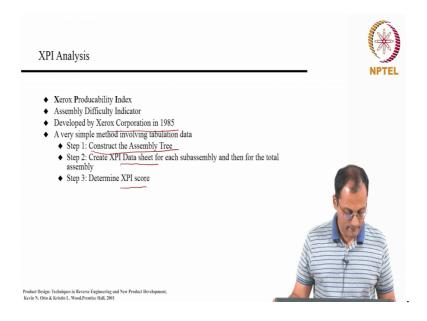
So, we create this assembly difficulty index. Just a small historical note, so developed by the Xerox corporation in 1985, when they were trying to optimise their assembly operations. The first step we have seen, we have created the assembly tree, the data that we have obtained regarding the attributes of assembly we will populate it into a data sheet and then, use the lookup table to determine the XPI score, which is degree of difficulty up to in the assembly.
