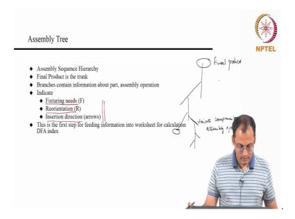
So, let us first see, how an assembly tree is created. I will take some example assembly and describe how an assembly tree is representative of the sequence of assembly operations that will go into the assembly.
