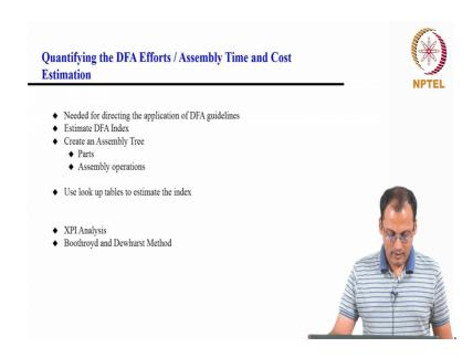
So, the index that can be used for assessing the assembly difficulty could be either the cost, which is essentially in terms of the assembly time. So, most of the methods tries to obtain an estimate for the degree of difficulty, in terms of the assembly time, which can then be converted into caste, based on the labour or based on the automatic assembly line setup cost and the operating cost of the assembly line setup.
