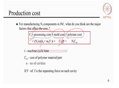
But the production cost is the total the cost since the number of components that are being made is more it will come down with multiple cavities. So, the total cost is processing cost, the mold cast and the material cost. So, the material cost is determined based on the material that is selected and it is not dependent on the number of cavities that are there in the mold, but number of cavities determines the mold cost and also the processing cost which is the hourly rate.
