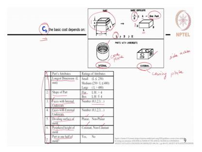
So, if I have a one part L, B and H are the dimensions of the part the largest dimension, L is a critical attribute so that is one of the first part attributes that we need to consider. So, all these part attributes are used with the table that we saw earlier to determine C b. The next attribute that we need to compute or infer is whether the part is flat or whether it is a box part so that is computed by seeing the aspect ratio of the basic envelope.
