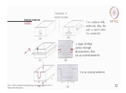
The external undercuts are these kind of features it could be either holes, it could be protrusions. This is not an external undercut as again we can see this is placed along with the parting line and thereby it can be made with the mold feature in the mould opening and closing direction itself. So, such features needs to be machined on the cavity side and thereby they are external undercuts.
