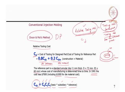
The mold cost estimation has been studied and documented based on several studies. We will look one such a method which is called as the Dixon and Polis method or in short as DP method. So, the cost of the part or the mold part is computed using a term called relative tooling cost. The relative tooling cost is given as tooling cost for the part divided by tooling cost for the standard part.
