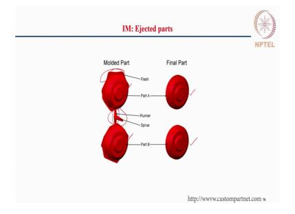
In the part comes out of the mold or when the part is ejected, there are few unwanted the elements associated with the part like the flash. A flash is required because flash ensures that the mold has completely filled and the material actually tries to come through the parting surface. This ensures that all parts of the mold are filled. So, flash is an essential component that can be minimized, but cannot be completely removed.
