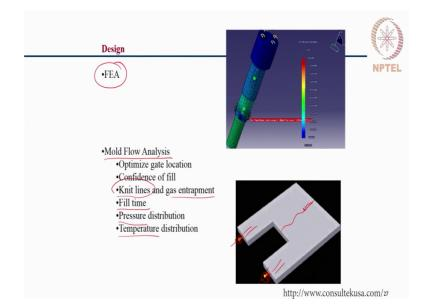
Another design tool which helps in proper design of the plastic components is using the numerical modelling and simulation using finite element method. One can also do what we call as a mold flow analysis. Analyzing how the mold flows into the material flows into the mold, the temperature distribution, the pressure distribution. All these can be studied numerically by computer simulation models.
