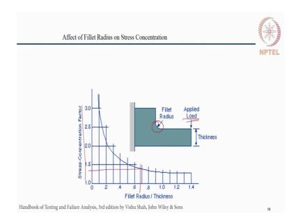
Studies which reflect upon how this corner radius will have an effect on this stress concentration. So, one can choose an appropriate radius and know what kind of a stress concentration factor, one has to use in the design for any given applied load.
