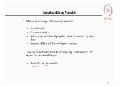
It can be used wherever there is chemical and corrosion resistance is required, where we need good strength, we can use it. And the limitations in terms of the usage comes from the fact, they cannot be used for very high mechanical loads and also for very high temperature applications. Typical usage temperatures are up to about 200 degree Celsius and there are some grades of plastics which can serve at slightly higher temperatures.
