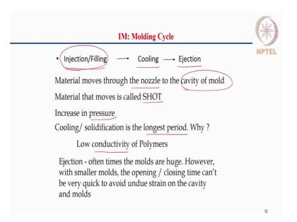
So, typically it consists of the filling stage or what we call as the injection stage and then, the part cools inside the mold and then the part is ejected. So, the material that is injected through the nozzle into the cavity of the mold is called as a short. And to make the material move into the mold, we need to increase the pressure.
