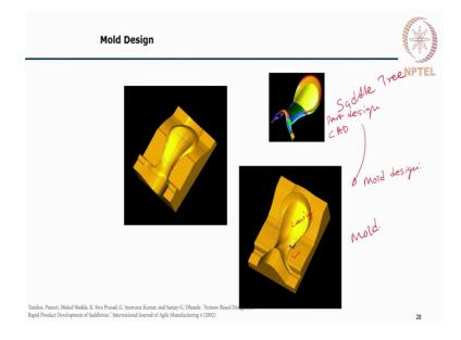
So, this an example design process, which I am showing using one product. This is called as a saddle tree which is used in the saddle which is main ha you know leather component used to help jockey sit on a horse while riding. So, this is a saddle tree which is a injection molded component what you see is a cad drawing. Based on the cad, one designs the mold.
