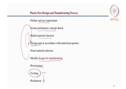
So, a plastic part design and manufacturing process starts with defining the end use requirement, because that decides the type of material that needs to be used and the process for manufacturing the same. Based on the functional requirement, preliminary concept is generated design concept is generated and material is selected and the part design is made according to that.
