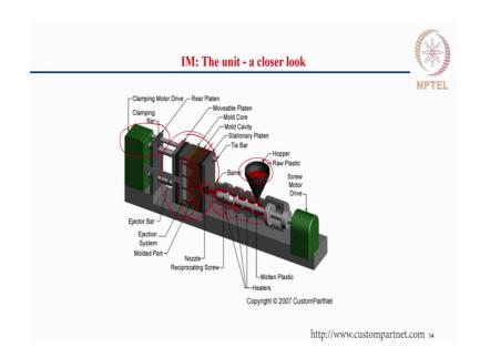
This is the mold and this is the injector. We have a nozzle here through which the material is injected this is a hopper from which the material is fed. So, there are heaters available in the injector, which heat the material and the material flows through this nozzle into the mold cavity.
