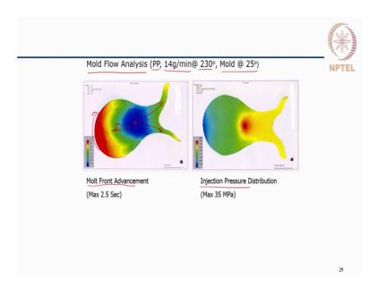
Once we have the mold design, we can use suitable software's to do the mold flow analysis like here you see a simulation of polypropylene being injected at 14 grams per minute rate at this temperature mole being kept at 25 degrees. It shows the mold front advancement how the material flows from the injection point.
