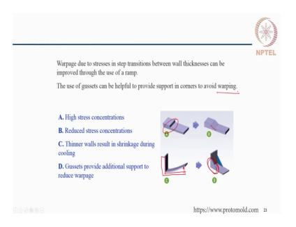
So, warpage can be avoided by providing gussets. So, these are the gussets without gussets the as designed component is supposed to be like this. But once the mold is done
