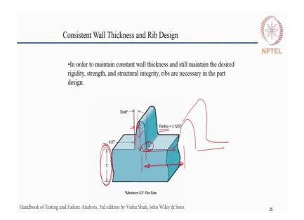
Ribs are to be designed properly. So, that one can avoid failures at these corners. So, one of the important feature dimension is this corner radius. Based on this nominal wall thickness T, one has to make appropriate choice of this radius the height of the rib and even the placement of the successive rib. Let us say if an another rib has to come here, what is the distance between the placement of two ribs?
