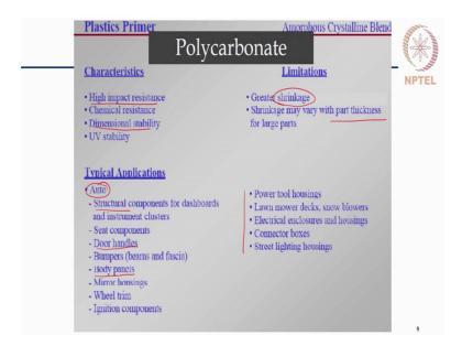
There are guidelines available for choosing the materials based on the various characteristics few sample materials, we will see. So, one of the most used materials is polycarbonate are or in short we call it as pc. It has very good impact resistance and dimensional stability apart from various other positive attributes is predominantly used in automotive structures wherever strength and impact resistance is important like door handles body panels etcetera.
