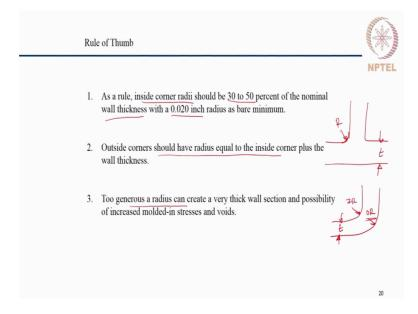
The general rule of thumb is to have an inner corner radius about 30 to 50 percent of the normal wall thickness say, the normal wall thickness is t a corner radius here R has to be about 50 percent of this value.
