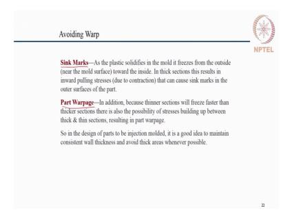
So, we as we saw sink marks are caused because when the plastic solidifies on the surface material is pulled inside and thereby the surface shows a sink mark. And part warpage is again due to shrinkage because largest section is shrinking it pulls a thinner section or deforms the thinner section because of the shrinkage of the larger section. So, these are typical problems associated with the plastic component.
