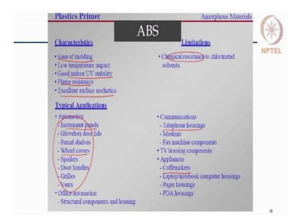
The other important materials is ABS. So, this is used primarily because of the excellent surface characteristics and ease of molding apart from several other characteristics like flame resistance and UV stability.
