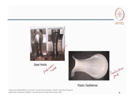
These are pictures showing the finally, manufactured tools. Once this simulations are done and the design of the mold is verified, one can go for production tools and we have the production parts coming from that. So, we see that the design of the mold is critical from the perspective that the material has to flow, we need to optimize the filling time or what is called as the mold cycle time. So, that the cast is kept at the minimum.
