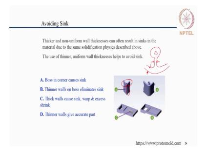
To avoid sink marks one can use uniform wall thickness as far as possible wherever it is not possible, one has to put design features that will help in maintaining uniform thickness. As we can see over here, there is a corner feature because of which there is a change in the thickness and causing the sink mark.
