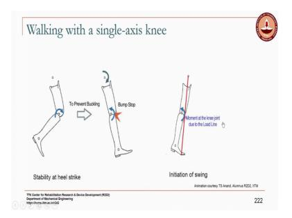
So, to prevent the buckling what the user does is they apply a hip extension moment which causes it to hit the bump stop, which causes the knee to lock by contacting the bump stop. And, that moves thee by moving that load line, it now generates an extension moment about the knee.
