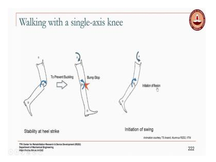
And now so, the user applies a flexion moment to shift the load line and initiate flexion. So, this is the working together of the how the user can use that residual hip moment or that normal hip moment to shift the load line in order to create extension or flexion at the knee in the absence of active control at the knee directly, because you are controlling the knee through the hip here ok. So, I just wanted to show you this animation.
