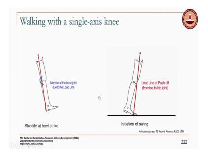
If the load line is behind the knee, then the moment at the knee joint will tend to make it buckle right.
