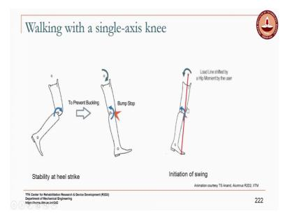
Now, in the case of push off, the moment at the knee joint due to the load line is an extension moment.
