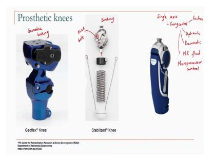
So, swing control can be, you can have friction you can have swing control using hydraulic or pneumatic units or now you also have knees that use MR fluid to control the swing face. Then of these some of them can be just mechanical hydraulic or pneumatic or they could be also microprocessor controlled they could be some level of microprocessor control in built into the knee to handle different situations.
