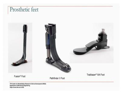
So, this one the heel shock absorption is only by means of these spring itself. So, these are all different, this is a multi axial foot the MA stands for Multi Axial. So, you could
