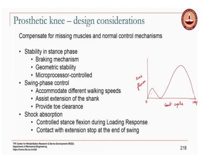
So, a person may actually become dependent on the braking mechanism and then suddenly one day it may it may have worn off to the point where it is not able to brake any more ok. So, where it is a geometric stability it arises out of the geometry of the linkage itself and so it is not subject to wear, with it does not change with time so it is more consistent.
