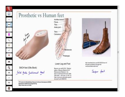
So, the simplest type of prosthetic foot is what is known as a SACH foot. So, SACH; stands for Solid Ankle Cushioned Heel, solid ankle cushioned heel is your SACH foot. And here you see on this side you see the Jaipur foot and you also see a cross section of the Jaipur foot. So, it has like a wooden block and some different types of rubber ok. So, you can see here.
