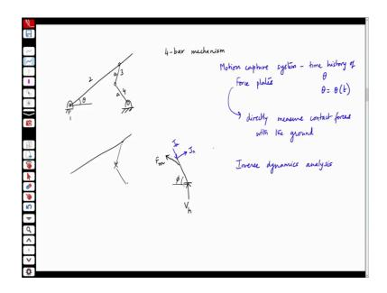
So, if you look at this model of the person doing the pushup, then I can equate it to do you recognize this mechanism? It is essentially a 4-bar mechanism ok, my 4 links are the fixed link, 2, 3 and 4. So, it is like four links pivoted together so, what is that tell me, so this is basically a 1 degree of freedom system then. So, if I know theta, I know the lengths of these two arms, so I know basically the orientation of these two.
