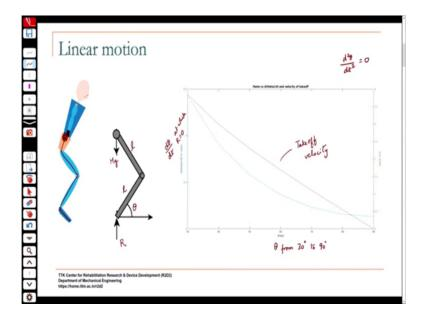
What at what d theta by dt the reaction force becomes 0? So, say theta I varied theta, theta from 30 degrees to 90 degrees in this simple model, and then I computed d theta by dt in radians per second at which r becomes 0 so, at take off ok. And then I computed the corresponding take off velocity, using the equations that we derived that ok.
