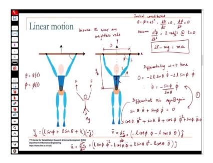
We will move on to linear motion will come back to this one. So, this is essentially the case that we did initially, where I told you that the acceleration of the center of mass is measured to be some value and we just computed the reaction forces ok. But if you look at how the human you know we are essentially influencing the motion of the center of mass by the movement of our arms.
