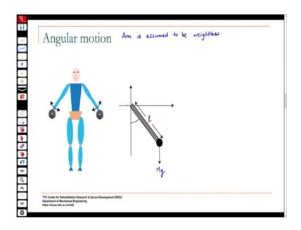
We will now move on to angular motion. And before we do that; so, in angular motion you also have the principle of angular momentum will also come into play in addition to Newtons laws, which tells you sigma f equals m times the acceleration of the center of mass ok. We will also have to consider the rotational aspects of the motion and we will look at the angular momentum principle for that.
