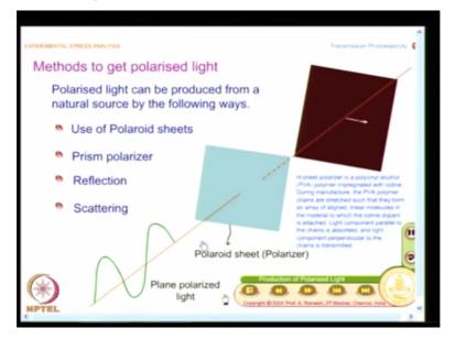
And first look at what is polarization. So I have a natural light, which is so random the magnitude as well as direction keeps on changing and the moment you put a polaroid sheet, you have a plain polarized light coming out after the polaroid sheet and this is only a statement and what I have attempted to show in this course is for any statement I make I try to provide you some kind of an experimental justification.
