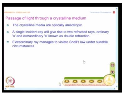
And what you have here? What happens when light passes through a crystalline media? First observation is the crystalline media are optically anisotropic. So how do you define isotropy? If the property is same along all directions, then you call that as isotropic. If the properties of function of direction, then it is anisotropy. So the first observation is crystalline media or optically anisotropic.
