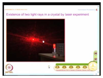
I will see the experiment so what I have here is I have this crystal is moving. Crystal is getting rotated. I have laser beam and I will replay this okay. What you have to see this is, I have a bright spot here and what you have to look for is when I rotate the crystal, you will see 2 dots and merge into 1 dot. See when the light is coming out of the crystal then they will interfere.
