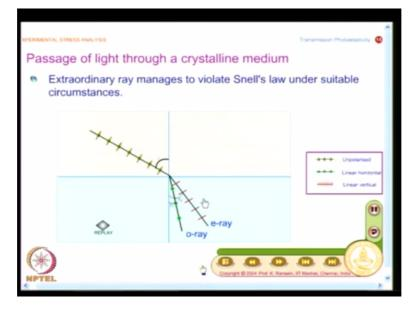
We will just look at the ray diagram and what happens here. So I have medium one and medium 2 now is crystal. It is not an isotropic media, medium 2 is a crystal and you draw the diagram, make a neat sketch of it, take your time and I can replay how the rays come. So I have a ray which impinges on this. Carefully look at how the incident ray is drawn and how the refracted rays are drawn.
