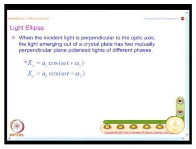
We will continue it in the next class, but this is what we will have a look at it. When the incident light is perpendicular to the optic axis, the light emerging out of a crystal plate has 2 mutually perpendicular plane polarized lights of different phases. This is what you have to understand. They have different phases is very important and you represent the light waves like this.
