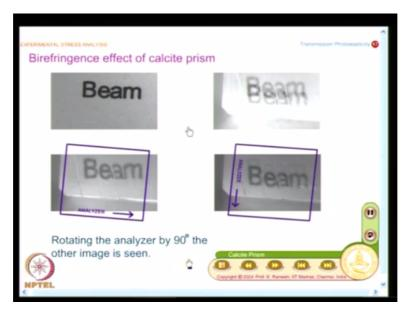
This is exactly so, so you could see here, I have 2 images seen, and you could also see, there is a slight shift. The shift is same as like what you see here. This is the image on the top and this is the image of the bottom. So I could filter out from this one of the images by employing an analyzer. So this shows that the beams are polarized.
