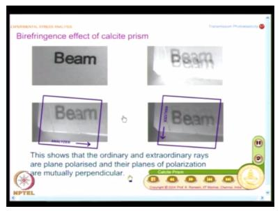
And because I get these 2 images when I keep them at mutually perpendicular positions of the analyzer, we also have established that these 2 beams are polarized in mutually perpendicular direction so that is what is summarized here. The ordinary and extraordinary rays are plane polarized. How do you establish they are plane polarized? I just use an analyzer, which would only cut off light perpendicular to it.
