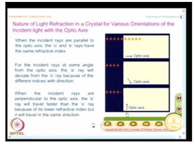
And now what we will have to look at is what is the direction of incident of light, which is suitable for photoelastic analysis and when you take a crystal, you have what is known as optic axis. I have a crystal here and I have a ray of light impinging on it and how is this ray shown? This is an unpolarized beam, you have a dot and a straight line and if this direction is parallel to optic axis what do I find?
