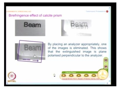
So what I will do is I am going to put a polaroid sheet on top of it and the intermediate process is not shown, final process is shown here. So I have analyzer and I oriented in this direction, what do I see? I see only one of the images what I saw as 2 in the earlier case. So this goes to prove 2 things, you find these rays are polarized that is why I am able to cut off one image.
