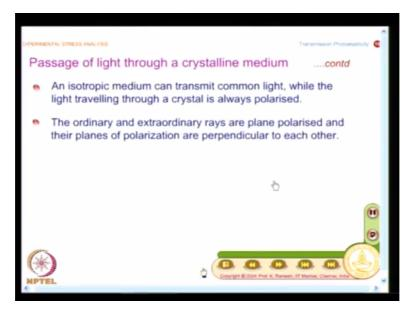
And we summarize these points. The first point is an isotropic medium can transmit common light, which is nothing but natural light. So an unpolarized beam will go as unpolarized beam while the light traveling through a crystal is always polarized. This is a very key and important point. So within a crystal whatever the light that travels through, it is polarized. A crystal cannot sustain unpolarized light.
