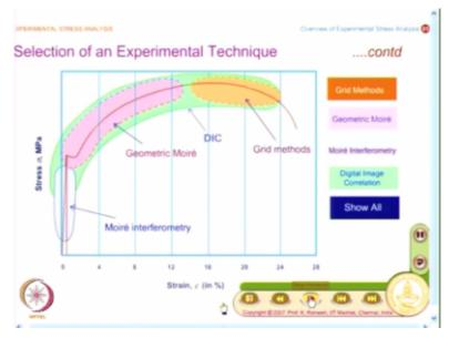
I have grid methods, I have digital image correlation, I have geometric Moire and I have more interferometry, so this gives you a reasonable appreciation on how to decide the techniques based on the strain range.
