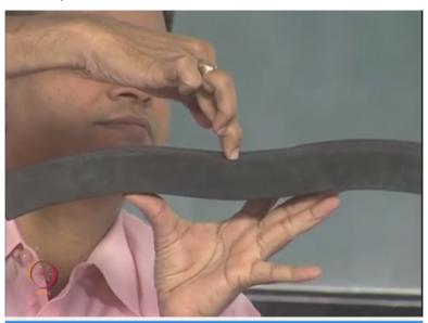
And then the next problem is you know; essentially you have to find out the shear distribution on a 3-point bend specimen, suppose I have this as the beam and I have supported like this and I put a sharp load like this now, what I need to do is from your strength of materials, if I want to find out the shear distribution over the depth, what is the variation? It is a parabola okay but what will be the variation when I come closer to the loading point.
