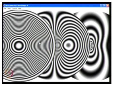
And here you find the use of techniques like Moire, holography or shearography to reveal various fringe patterns and you find here this as the out of plane displacements. Now, you know that this is the slope, this is the curvature information and each of this requires separate optical arrangements and you may be able to get this displacement by the technique of holography or speckle interferometry or shadow mining.
