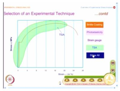
And thermo elastic stress analysis is proposed as a whole field strain gauge technique, that is how they are propagating the technique now and you can go from elastic to plastic region and this is more of a whole field representation but the instrumentation is very expensive, understand that. Strain gauge instrumentation is lot more simpler when you compare it to TSA but even that instrumentation is costly, it is not cheap and now you have a relative zones for different techniques shown.
