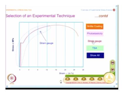
So, that means almost close to 0 and you can also go to the plastic region about 10, 12% of strain, you can easily measure with strain gauges. So, you can also understand why we say strain gauge is a versatile technique, so it has a longer range I can go from elastic to plastic comfortably.
