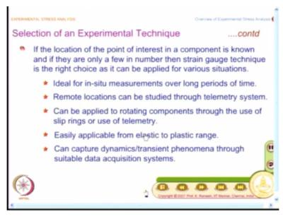
Then you also have to look at what is the thoroughness of the study required and finally the cost permissible for the study that is also equally important. Then what we looked at was; if the location of the point of interest in a component is known a priori and if only a few in number, then strain gauge technique is a right choice as it can be applied to various situations and one of
