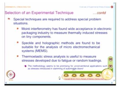
So, a combination of hole field and a point by point technique they go together and they help you to solve the problem, so day to day design problem you can handle and also in special situations. So, you can always fall back on either photo elasticity or strain gauges. For special situation what you have to do? You have to go in for special techniques, so you need special techniques to address special problem situations.
