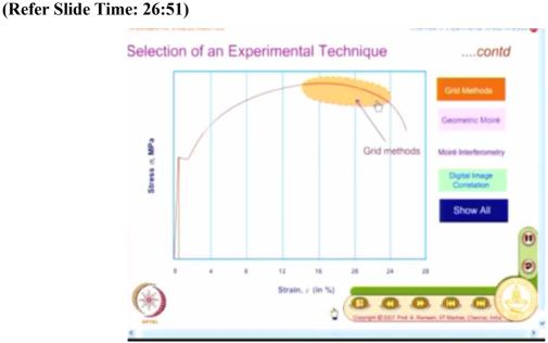
They are grid methods, geometric Moire, Moire interferometry, digital image correlation and you know grid methods were the one, which is used for very high plastic region, then you have geometric moiré and Moire interferometry is refinement of geometric Moire and digital image correlation. It has a large range but it does not have accuracy at lower strain levels. So, when you look at grid methods, the range is somewhere here.
