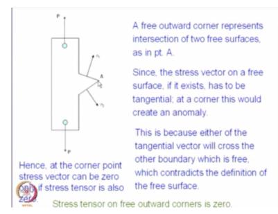
I have a projection like this and I am not interested in finding out stresses at all these points, I would like to know what is the stress magnitudes at the sharp corner, a. Can anybody say? When I have a sharp corner like this, suppose instead of this corner I have a corner which is like this, I have a cut out here then it lacks like a v-notch and you have singularity at the crack tip at the angle and so on, you call that as re-entrant corner.
