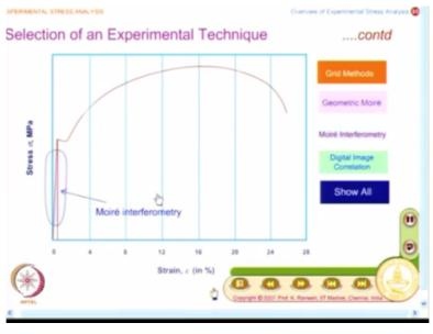
The issue here is what is the range of strain that you are really looking at and Moire interferometry cannot measure very small strains, it can go down but it cannot go close to 0 and these are you know pictorial representation; numbers are not given, so you find that this is the range that you are really working with Moire interferometry.
