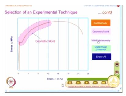
It is only in the highly plastic region, you have the grid methods are applicable and when you come to geometric Moire, I would have it somewhere here, this is how I will be able to do this and if I want to lower this, then I can go for Moire interferometry and what you need to worry about is this end point and start point. This shape is for convenience, for aesthetic beauty some shape is drawn.
